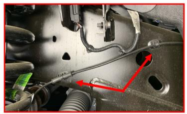
Connect the CCD solenoid harness connector.
