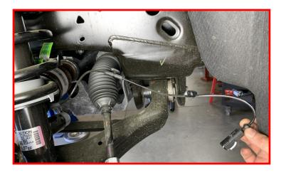
Install the (2) retaining clips that secures the CCD solenoid harness to the frame.
