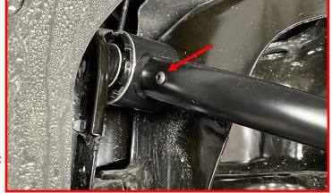
NOTE: IF INSTALLING KIT ON A VEHICLE EQUIPPED WITH AUTO ADJUSTING HEADLIGHTS OR CCD INSTALL THE SUPPLIED UPPER CONTROL ARM CLAMP USING THE SUPPLIED M5 ALLEN BOLT.
