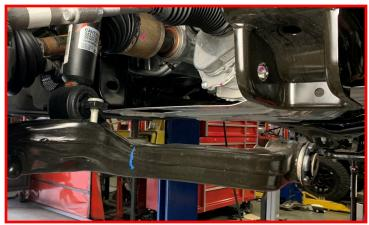
NOTE: USING A MARKING DEVICE LIKE A PAINT PEN, MARK THE STRUT AT THE OUTBOARD POSITION. THIS MARKING WILL BE MOUNTED INBOARD DURING LIFTED STRUT INSTALLATION.
