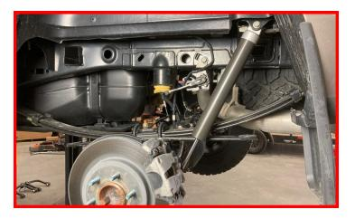
Prior to installing wheels, complete all installation steps on the opposite side. Install the wheels and lower the vehicle to the ground. Torque the lug nuts to the wheel manufacturers specs. Jounce the vehicle to settle the suspension to the new ride height. Torque the lower control arm hardware to 200 ft-lbs and rear shock hardware to 75-ft/lbs.
