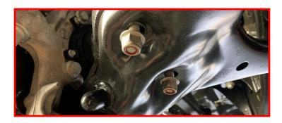
Loosen and remove the lower control arm pivot bolts. Retain the factory bolts.
