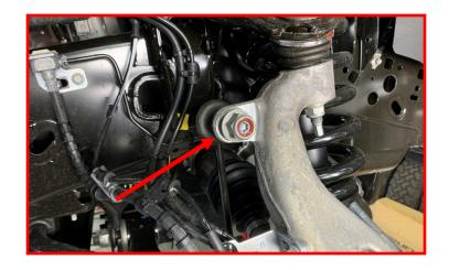
Using the appropriate tool, grease the upper ball joint until the boot just starts to expand. Do not over grease. Over grease can cause pre-mature wear.
