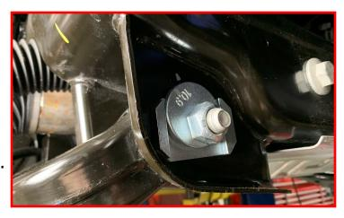
Tighten the top strut nuts.
