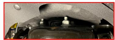
Remove the lower strut nuts. Retain the factory mounting hardware.
