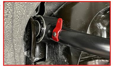
Install the front sensor ball stud into the upper control arm clamp using the factory hardware.
