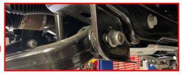
Remove the lower control arm pivots from the frame side pivot pockets.
