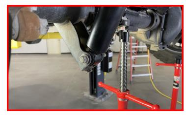
Install the supplied Falcon rear shock using the factory hardware. Torque after reinstalling the wheels and lowering the vehicle to the ground.
