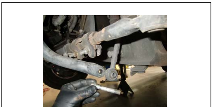
Remove the bolts and twist the sway bar out of the way.
