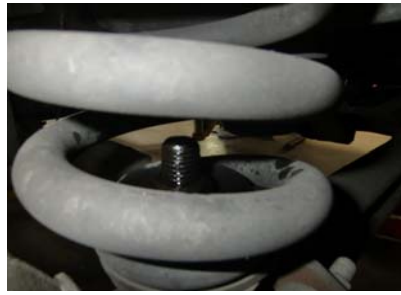
Remove the nut and washer.
