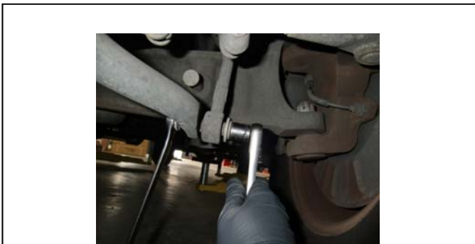
Unbolt the sway bar on both sides of vehicle.
