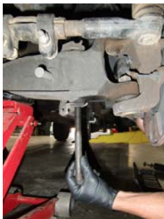
Remove the bolt between the radius arm and beam.
