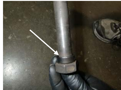
Place the spacer over the bolt.
