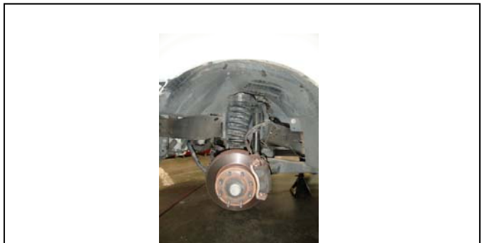
Lift the vehicle off ground and remove the front tires.
