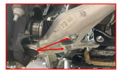
Remove the lower control arm pivot nuts from the frame side pivot pockets.
