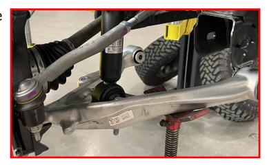
Continue to raise the lower control arm up until the strut studs are exposed enough to install the factory mounting hardware.
