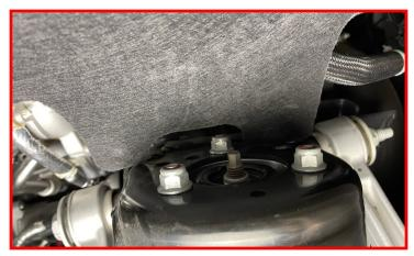
Remove the lower strut nuts.
