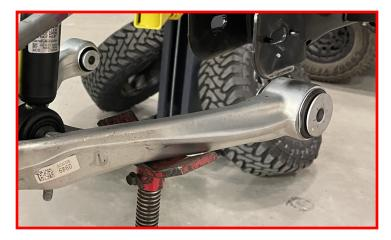
Install the factory alignment cam plate over pivot bolt and then install the nut.
