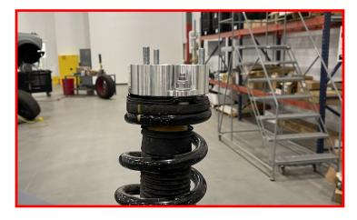
Using the supplied M10 nuts, install the completed strut assembly into the frame.
