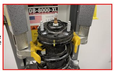
To aid in the installation process, clamp the lower strut stud in a set of soft jaws. Using the leverage of the strut, rotate the lower strut bushing about 30 degrees in the opposite direction orienting the lower strut studs parallel to the strut body.
