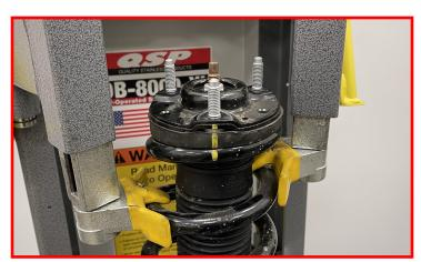
Compress the spring enough to relieve pressure on the top hat. Being sure to keep the strut body and upper spring isolator in the factory location, rotate the factory top hat 180 degrees from the previously made marks. This will orient the spring in its original location to prevent the spring from bowing.
