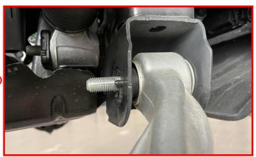
Remove the lower control arm pivot bolts. Retain the factory hardware.
