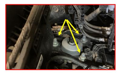
Loosen the upper control arm bolts to relieve the preload on the bushings.
