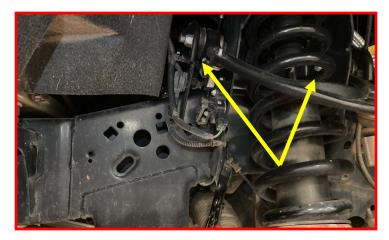
Remove the tie rod nut at the knuckle. Use a dead blow or similar to strike the face of the knuckle to remove the tie rod end.
