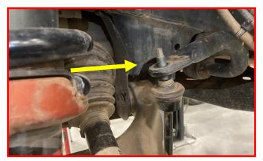
Support the knuckle at the lower ball joint and remove the lower control arm bolts.
