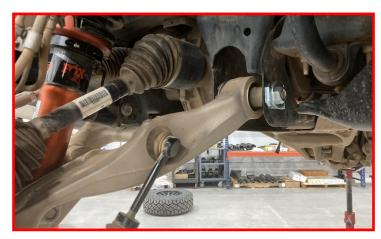
If using ReadyLIFT P/N 86250 Cam Kit, install the cam washer over the bolt so that the alignment pin on the washer seats into the hole on the frame.
