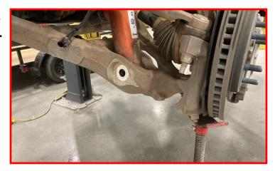
Remove the three upper shock mounting nuts.
