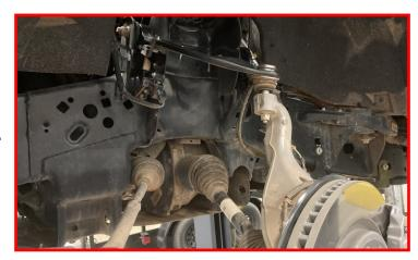
Remove the Live Valve wire from the lower spring perch
