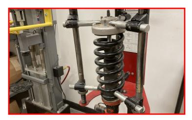
Using a rubber mallet or similar, slide the lower spring perch up the shock body to remove the factory spring perch retainers.
