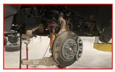
Support the shock and spring and remove the lower shock bolt from the control arm.
