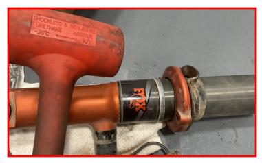
Using the groove in the shock body, Install the ReadyLIFT pre-load spacer.
