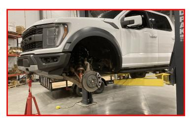
If equipped, unplug the live valve wire and remove plastic clips from frame
