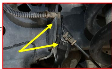
Remove the nut holding the shock to the lower control arm.
