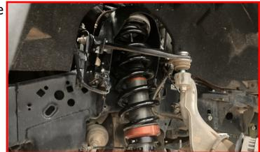
Simultaneously insert the lower shock into the mount as the control arm is fitted to the frame mounts.
