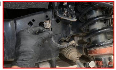
Loosen but do not remove the three nuts at the upper strut mount.
