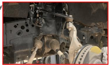
Install the supplied clip and mount the live valve wire to the new pre-load spacer using the supplied bolt.
