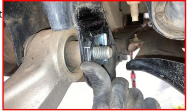
Install the lower control arm nut.
