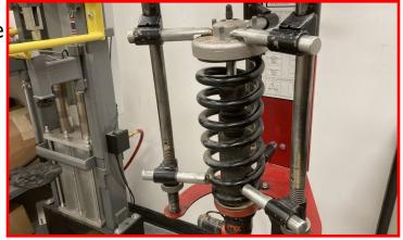
Install the shock assembly by replacing the three factory upper strut mount nuts.
