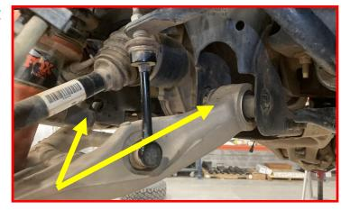
Rotate the control arm toward the rear of the vehicle and gently let the arm hang from the frame.
