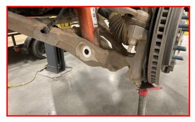
Reinstall the sway bar link using the factory nut.
