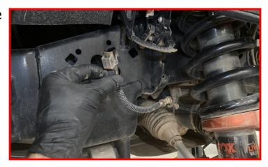
Free the Live Valve wire from the frame completely.
