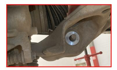
Remove the sway bar link from the sway bar.
