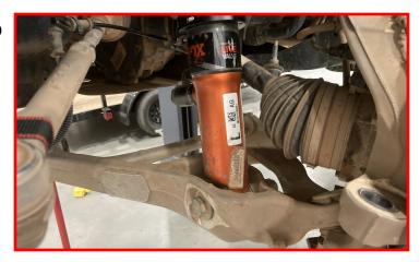
Install the lower shock mount bolt and lower control arm bolts.
