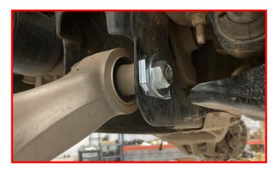
Reinstall the tie rod end using the factory nut.
