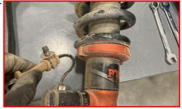
Using a spring compressor, separate the shock and spring.
