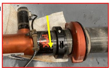
Align and seat the lower perch on the ReadyLIFT pre-load spacer and reassemble the shock, spring, and upper spring perch assembly using the factory nut.
