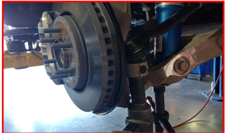
Install the brake line bracket to the knuckle using **factory hardware**. Torque to **5 ft-lbs**. Install the ABS line back to the frame, to the rubber brake line clamps, and knuckle using **factory hardware**. Torque to **165 in-lbs**. Install the vacuum lines to the vacuum actuator.
