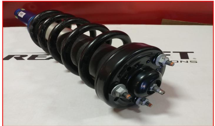
**1.5" kit top extension only:** If you are only installing the top extension kit, Put the strut assembly into a suitable spring compressor and release the tension. Rotate the factory top hat **180 degrees** from the factory orientation using the previous marks made as a guide. Remove the strut from the compressor.
