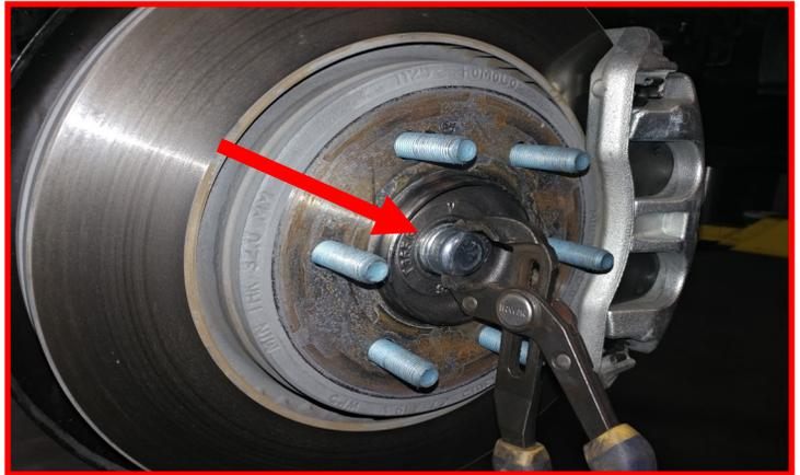
Remove the CV axle nut.
