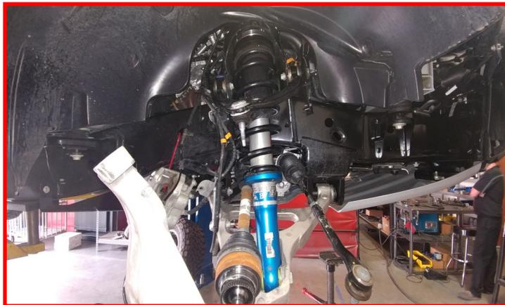
Raise the lower control arm up while guiding the axle and lower strut into place. Install the lower strut mount **factory hardware**. Do not tighten at this time.
