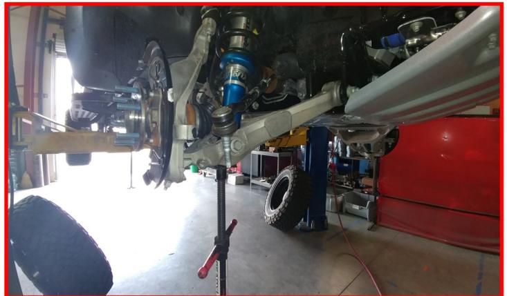
Lower the upper control arm while lining the upper ball joint into place. Install the upper ball joint to the knuckle using **factory hardware**. Torque to **65 ft-lbs**.
