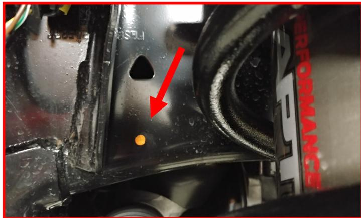
Route the coil over harness up along the control arm sensor harness on the frame rail and behind the plastic wheel liner using the factory clips along the way. Plug the electrical connector back in.
