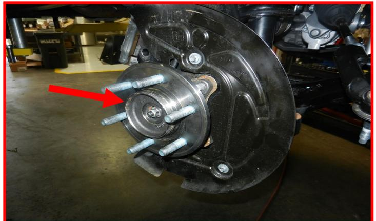
Jack the lower control arm up to add pressure to the strut. Putting a suitable jack stand at the rear of the vehicles frame will aid in keeping the load transfer from picking the front end up while jacking the lower control arm up.
