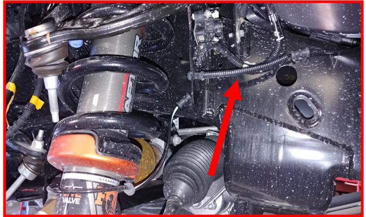
Disconnect the electrical connector and remove all clips from the frame rail.
