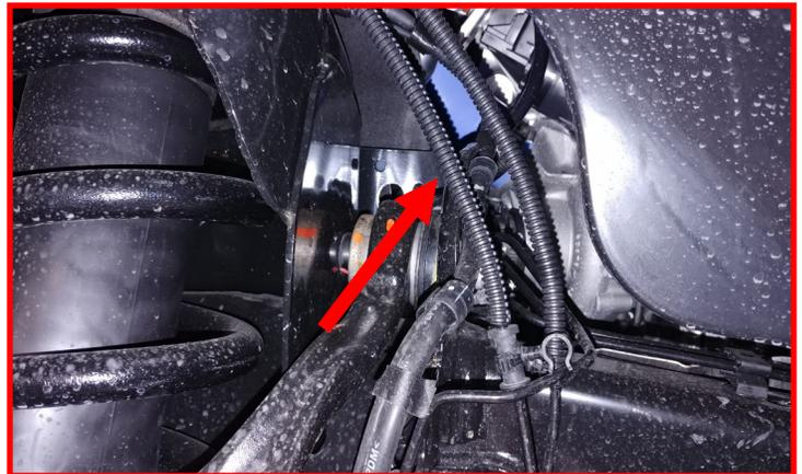
Disconnect the electrical connector and remove the wire from all other points on the frame. Picture is of the top of the inner fender well plastic showing the harness clip for the electrical connection. This can be accessed from under the hood or reaching up behind the plastic. Remove this clip from the plastic liner as it will need to be relocated in a later step.
