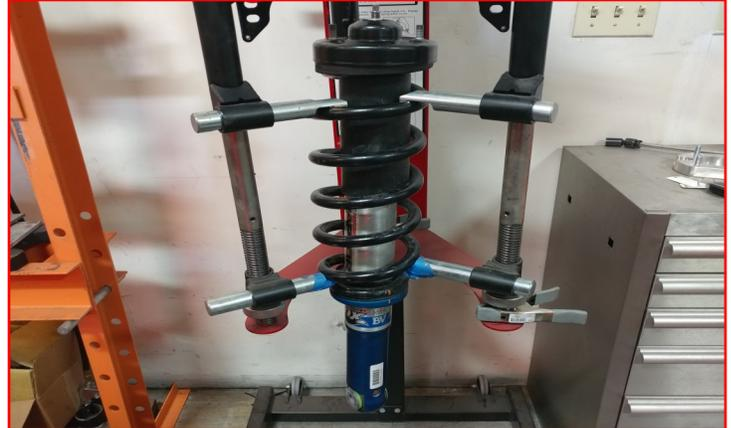
**1.5" and 2.5" kit top extension:** Install the factory nuts onto the strut hat studs running them down until they bottom out. Using a suitable cutting tool, cut the studs off just above the nut. Remove the nuts and clean any off any burrs. Paint the exposed metal with a quality rust preventative paint.
