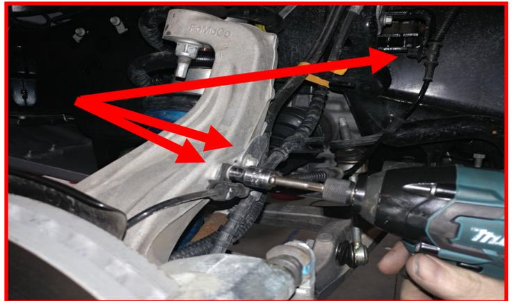
Remove the vacuum hose from the vacuum actuator on the knuckle.
