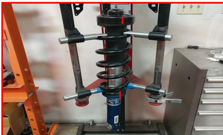
**2.5" kit Spring spacer:** Remove the factory top hat. Pull the rubber isolator and dust shield out and replace onto spring.
