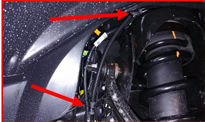
Mark another hole location in the plastic wheel liner in line with the original mounting hole but on the lower portion closest to the engine bay. Use a 7/16" drill bit and suitable drill to make the hole. Make sure to only drill through the plastic liner and not anything else. Move any wire harness that may be in the way to drill the hole. Install the coil over electrical connector clip into the new hole.
