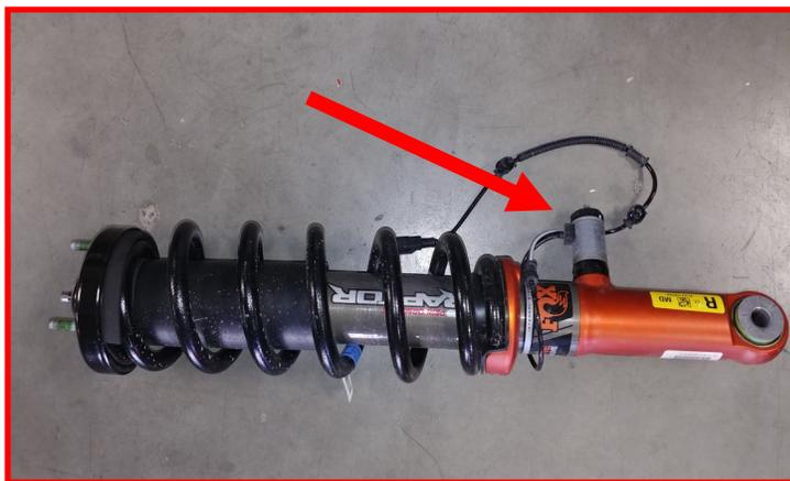
**2.5" kit Spring spacer:** Using a suitable spring compressor, release the tension on the factory top hat.
