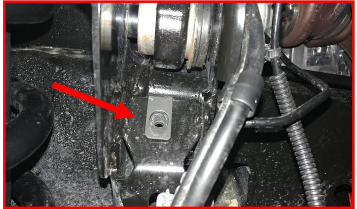
Install the ReadyLIFT provided **urethane bump** stop by screwing into the capture nut until fully seated.
