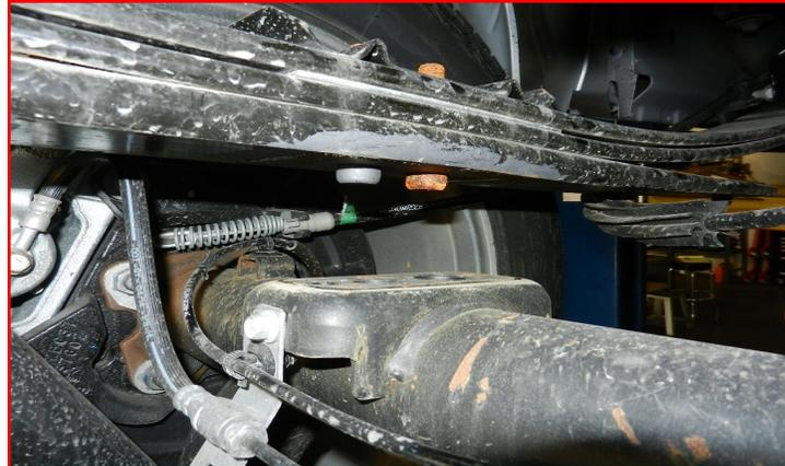
Locate the passenger side lift block, making sure the tapered end points to the front of the vehicle. Install the lift block on the axle pad aligning the pins. Raise the axle and the block up to the spring while aligning the center pins. Install the provided **u-bolts, washers and nuts**. Snug the U-bolt nuts but do not fully tighten at this time. Repeat steps for driver side. Lower the vehicle to the ground and torque the U-bolts to **110 ft-lbs**.
