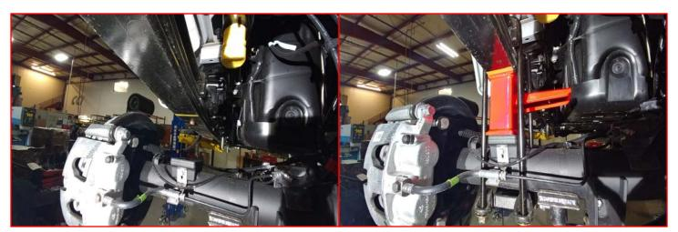
Install the ReadyLIFT passenger side block (if tapered, make sure the taper goes towards the front of the vehicle) (make sure the offset pins locate the axle to the front of the vehicle) and raise the axle lining the center pins up. Install using the provided u-bolts but do not fully tighten at this time. Repeat steps for the drivers side.
