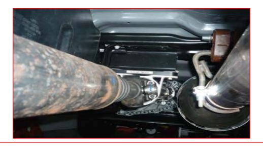
If equipped with a 2 piece driveline, remove the bolts holding the carrier bearing to the frame. Install the ReadyLIFT carrier bearing spacer between the carrier bearing and frame using 7/16" hardware. Torque to 50 ft-lbs.
