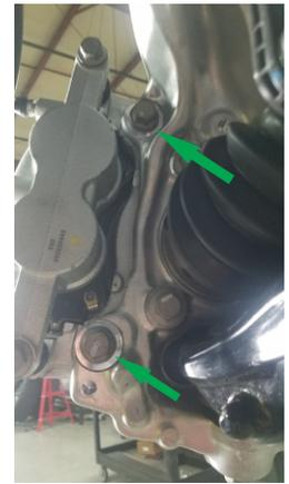
Reinstall the **ABS and brake lines** to the steering knuckle.
