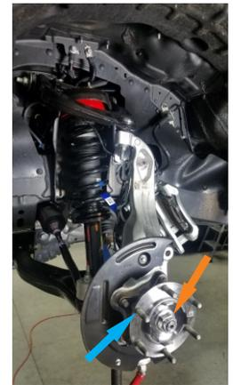
use a hammer to **dislodge the axle** from the wheel bearing. Use caution with this, don't strike the axle with the hammer. use a center punch and align with the center hole on the axle.
