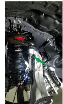
Reattach the **tie rod** to the steering knuckle, and tighten **45ft-lbs** of torque.
