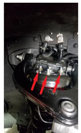
Using a jack raise the LCA and reinstall the bottom **studs of the strut** to the LCA hand tighten only.
