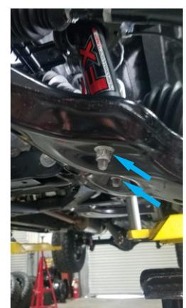
With the **upper ball joint** nut loose and the **tie rod** nut removed, strike the ball joint boss with a dead blow hammer to dislodge the taper. Once the taper is dislodged remove the upper ball joint hardware, and separate the UCA and the tie rod from the steering knuckle. Allow the steering knuckle to lean out, for clearance. Take care to not over extend or stretch the **CV axle** Adjust as necessary.
