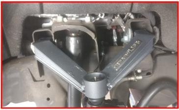
Install the upper control arm ball joint to the factory knuckle using the provided hardware. Torque to 85 ftlbs. Grease the upper ball joint using a high quality ball joint grease. DO NOT over grease. Install the Ready-LIFT ball joint cover by pressing into place.
