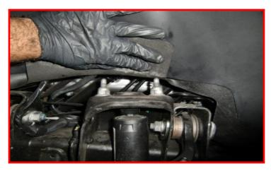
Remove the factory torsion bar adjusting bolt. Use a torsion bar unloading tool to relieve the pressure on the cross pin. Take care as the torsion bar is under extreme pressure. Always wear safety equipment.
