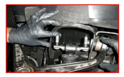
Install the shock back to the frame using the provided hardware. Torque to 30 ft-lbs. Install the front wheels and lower the vehicle to the ground. Torque the lug nuts to the wheel manufacturer's specs.
