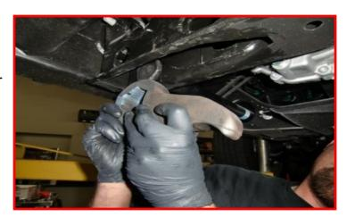
Install the ReadyLIFT keyway into the cross member while sliding the torsion bar into place. The tang of the keyway will be clocked slightly lower than the factory key. This accounts for the lift. Do not load the cross pin or bolt adjuster at this time. This will be done as one of the last steps in the front install.
