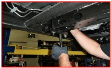
Install the shock spacers to the factory studs.
