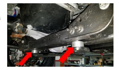
Trim the plastic gravel guard. Cut a slot just large enough for a 3/8 bolt to slide freely, on the lower mount that connects the gravel guard to the skid plate. Use the provided spacers large washers and bolts to attach at the lower mount. Hand tighten only. Use the factory hardware to attach the top of the gravel guard in its original position. Torque all bolts to 25ft-lbs.
