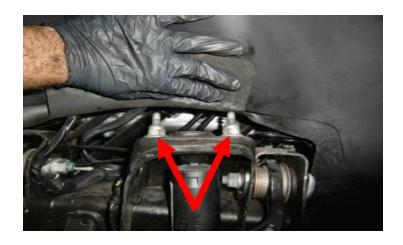
Add shock spacer to the upper mounting studs. Reinstall the shock to the upper mount. Use provided hardware torque to 45ft-lbs.
