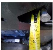
Install the differential skid plate. Install the two rear mounting spacers, large washer, and bolts. Do not tighten at this time.
