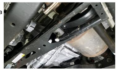
Factory torsion key part# 84461807 Screw in the torsion key adjuster bolt in until the measurement recorded on page 6 step one. Screw in the adjuster bolt an additional 3/8"
