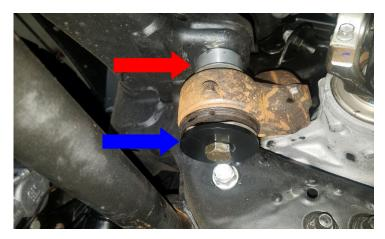
Loosen but do not remove the lower control arm bolts. This step is necessary to relax the bonded bushings for the new lift height. These bolts will be retighten when the kit is finished installed and the vehicle is on the ground.
