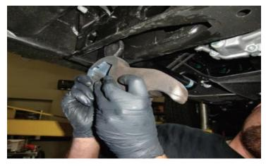
Install the ReadyLIFT keyway into the cross member while sliding the torsion bar into place. The tang of the keyway will be clocked slightly lower than the factory key. This accounts for the lift. Do not load the cross pin or bolt adjuster at this time. This will be done as one of the last steps.
