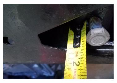
Install the differential skid plate with the rear mount only at this time. Use supplied M10x35 bolts, M10 fender washers and 1/2" spacer. Hand tighten only.
