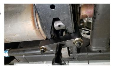
Remove the torsion bar unloading tool. Install the keyway adjustment bolt using a dab of grease on the threads and tip.
