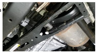
Factory torsion key part# 84461807 Screw in the torsion key adjuster bolt in until the measurement recorded on page 6 step one. Screw in the adjuster bolt an additional 3/8"
