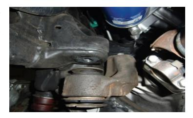
Install the ReadyLIFT differential spacers between the differential cradle and frame. Use the provided M14x130 bolts and laser cut washers. Use factory flange nuts. Torque all to 95 ft-lbs.
