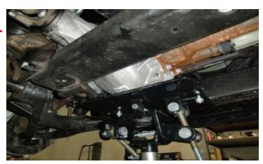
Locate the front and rear differential cradle bolts. (Total of four) Remove all and lower the differential down enough to install the differential spacers.
