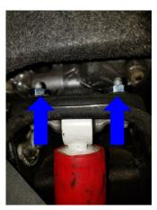
Measure and record the torsion key adjuster bolt length and part number. Remove the torsion bar adjustment bolt.
