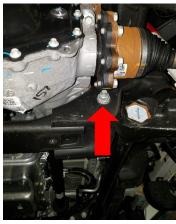
Use the torsion bar unloading tool, load the torsion bar enough to install the cross pin. DO NOT pull it through with your fingers.
