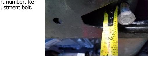
Using a torsion bar unloading tool (ReadyLIFT part #66-7816A or similar), relieve the pressure on the torsion key cross pin. Take care as the torsion key is under extreme pressure and can cause injury and/or death if handled improperly. Always use safety equipment.
