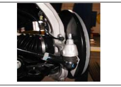
15. Reinstall the tie rods into the knuckle using a 21mm and 10mm wrench
