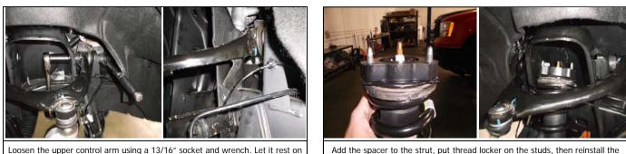
Add the spacer to the strut, put thread locker on the studs, then reinstall the the droop stop, then retighten the upper control arm and torque it strut into the vehicle. Use the provided hardware to mount the top of 12. the strut with a 14mm wrench.
