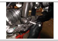
Loosen the lower control arms at the frame using a 24mm socket. Then 8. unbolt the strut from the lower control arm using a 21mm socket.
