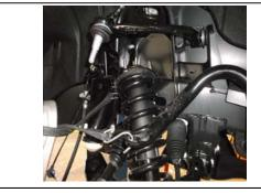
Lift the sway bar out of the way, then remove the strut from vehicle. 10.
