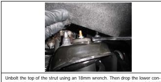
trol arm to make clearance for the removal of the strut. Note: DO NOT over extend the cv-axle joints, doing so will damage/ break them. q
