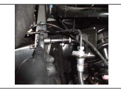
Remove the brake line bracket from the frame using a 13mm socket. 6.
