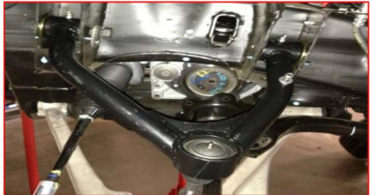
Install the ReadyLIFT upper strut spacer onto the strut. Rotate the bolt pattern until the spacer lines up.
