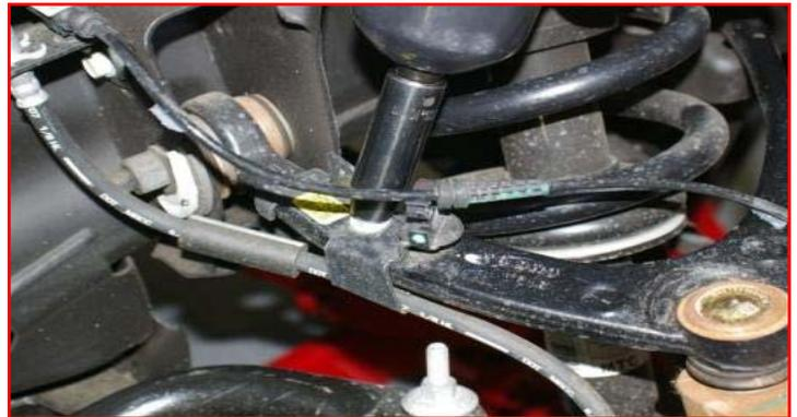
Remove the sway bar end links from the sway bar and lower control arm.
