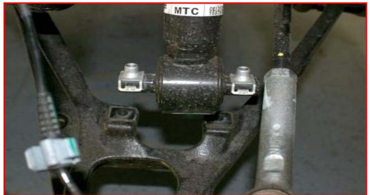
Remove the upper strut mount at the frame.
