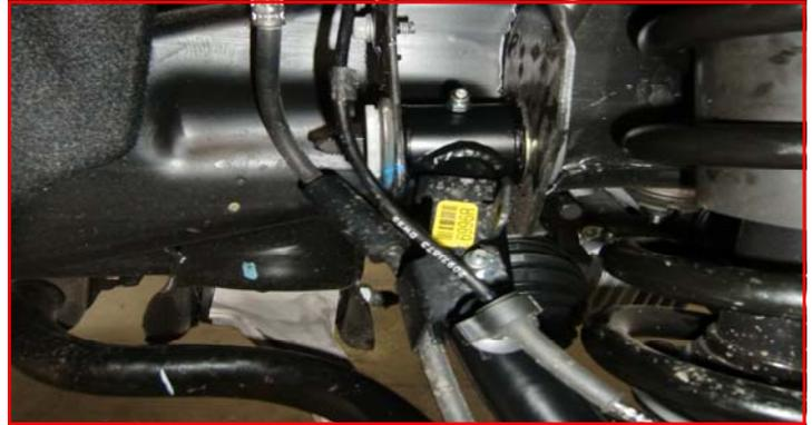
Attach the ABS wire to the frame rail with the factory clip. Re-connect the electrical connector.
