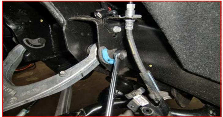
Install the appropriate side ReadyLIFT upper control arms into the frame using the **previously removed cam bolts and cams**. (New design control arms do not have Zerk fittings and do not require grease) Do not tighten at this time.
