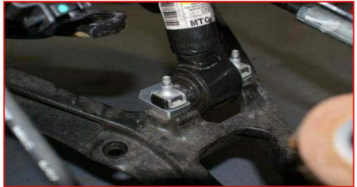
Install the sway bar end links and **factory hardware**. Do not tighten at this time.
