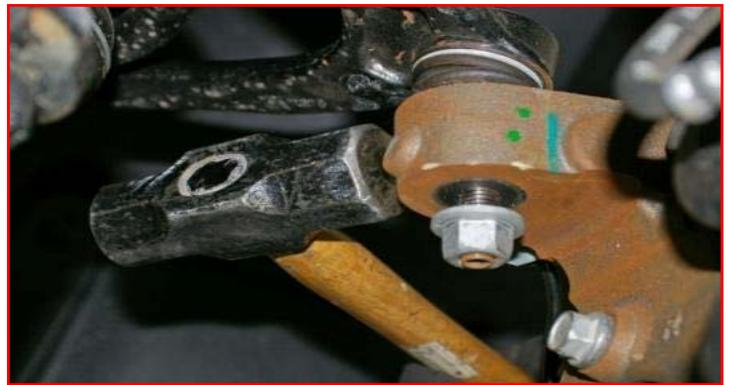
Remove the lower strut from the lower control arm.
