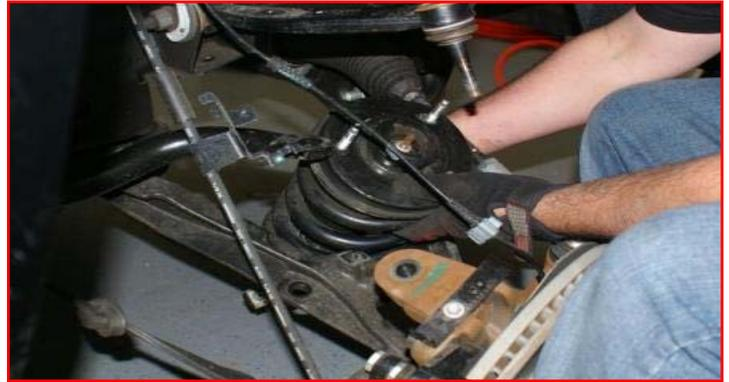
Remove the upper control arms. Make sure to note the orientation of the alignment cams for re-installation later.
