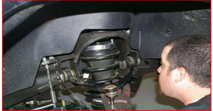
Raise the lower control arm and install the ReadyLIFT lower strut extension using the **factory hardware**. Torque to **45 ft-lbs**.
