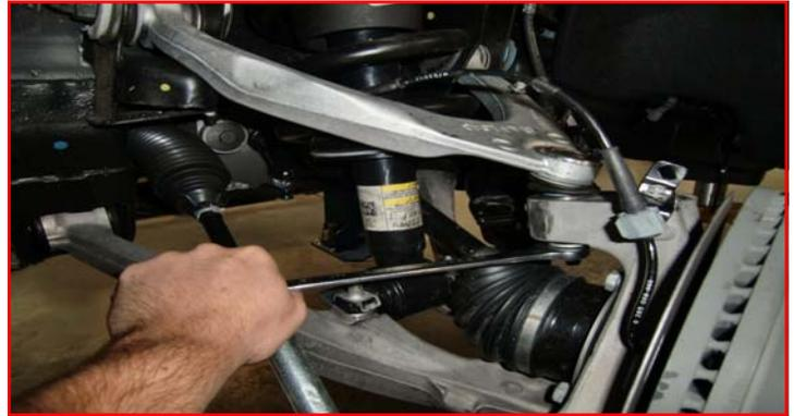
Strike the upper ball joint boss to release the taper.
