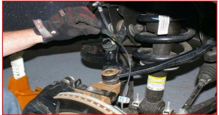
Remove the brake line bracket from the upper control arm and frame rail.
