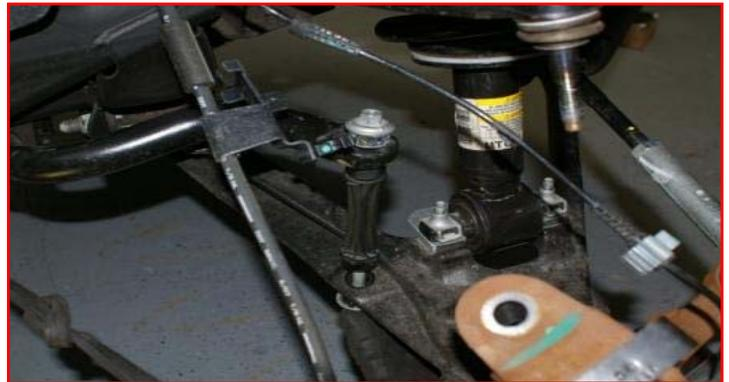
Attach the upper ball joint to the knuckle using the **provided hardware** (4wd guide the CV axle through the hub bearing while installing the upper ball joint). Torque to **85 ft-lbs**. DO NOT use an impact.
