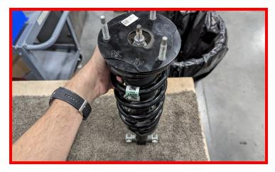
Install ReadyLIFT Strut Spacer.
