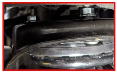
Install strut assembly to lower control arm bolts.
