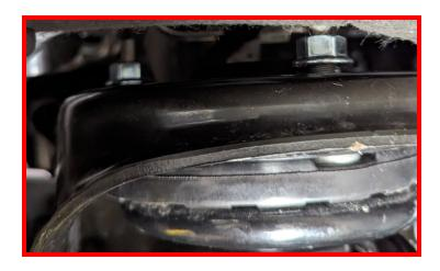
Tighten upper control arm to knuckle nut.
