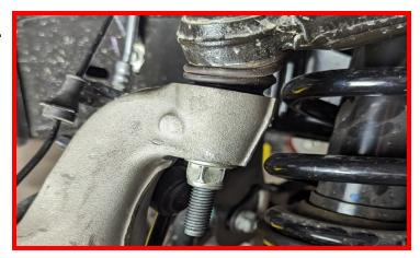
Install sway bar link into knuckle.
