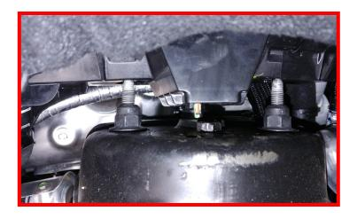
Loosen and remove tie rod nut and disconnect tie-rod from knuckle.
