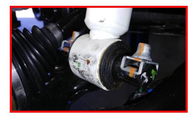
Remove sway bar link to knuckle nut and disconnect sway bar link from knuckle.
