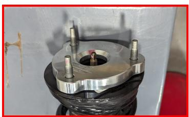
Using the supplied M10 nuts, install strut assembly into vehicle. Do not tighten at this time.
