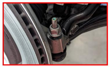
Torque strut top nuts to 35 ft-lbs.
