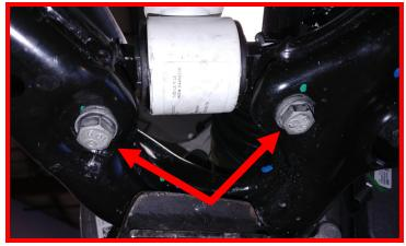
Tighten upper control arm to knuckle nut.
