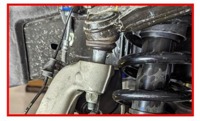
Remove strut assembly from vehicle.
