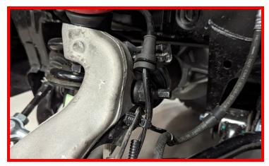
Loosen, but do not remove upper control arm to knuckle nut.
