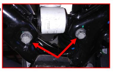
Install the factory nut on the sway bar end link. Torque sway bar end link lower nut to 45 ft-lbs.
