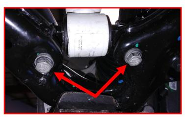
Loosen but do not remove the lower control arm mounting hardware. Locate the lower shock bolts and remove. The shock may "pop" outboard when removed due to the angle of the control arms.
