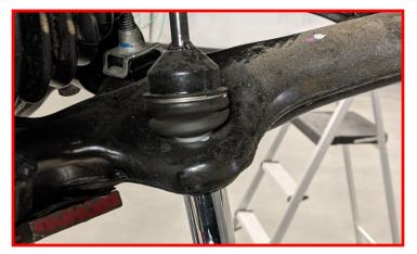
Using the factory nut, install the upper control arm into the knuckle. Torque upper control arm to knuckle nut to 65 ft-lbs.
