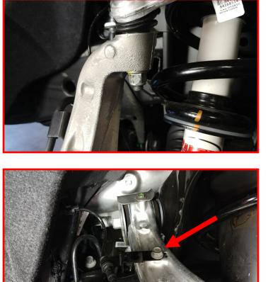
Install the brake line bracket from the upper control arm using the factory hardware. Torque to 5 ft-lbs.
