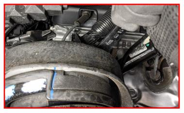
Torque shock to lower control arm bolts to 45 ft-lbs.
