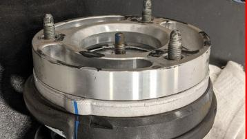
Re-install the shock to lower control arm bolts. Do not tighten. Using the jack under the lower control arm, raise the arm up until the shock studs are protruding through the frame holes in the shock tower.
