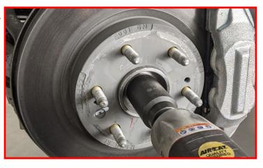
Using a dead blow sledgehammer, strike the end of the axle until it moves back and forth freely. Remove axle nut at this time, be sure to retain the axle nut for later installation.
