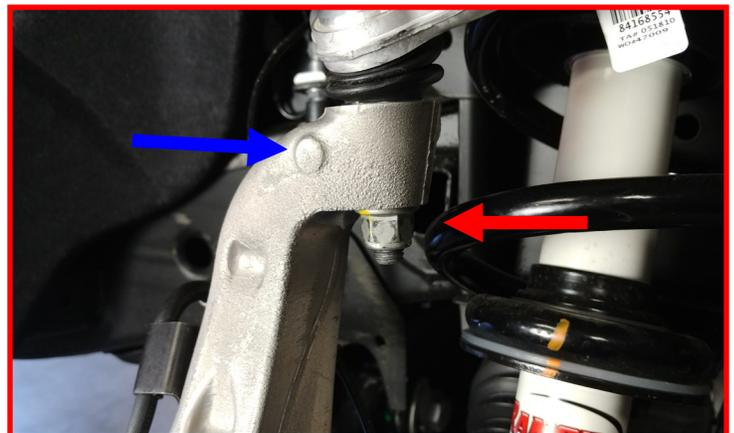
Loosen but do not remove the lower control arm mounting hardware. Locate the lower strut hardware and remove. Discard as they will not be reused. Lower the jack while applying pressure towards the frame rail on the strut body. Due to the length of the strut and angle of the strut tower, the strut will "pop" out towards the knuckle.
