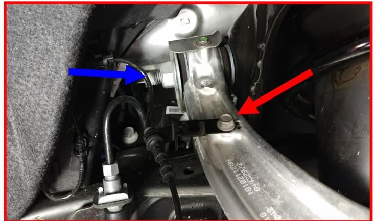
Loosen but do not remove the upper **ball joint nut**. Strike the **ball joint boss** with a dead blow hammer to dislodge the taper. Remove the upper control arm from the knuckle. Let the knuckle hang out of the way. Take care to not over extend the brake line and ABS wires.
