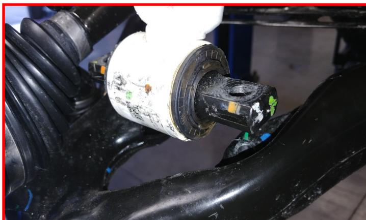
Install the ReadyLIFT lower strut extension in between the strut and lower control arm. The extension is tapered and will be installed correctly when the ReadyLIFT logo is legible from the engine side of the suspension.
