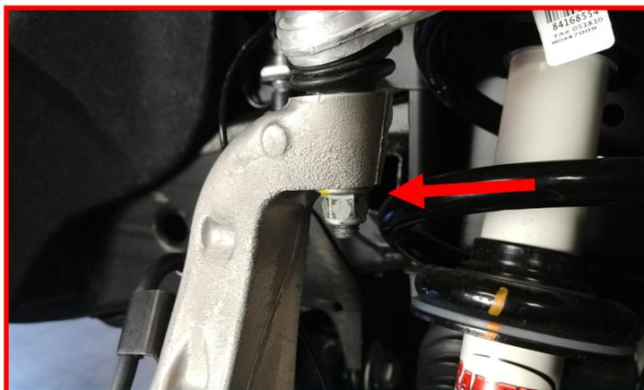
Re-attach the brake line bracket to the upper control arm using the **factory hardware**. Torque to **5 ft-lbs**.
