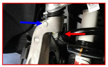
Loosen but do not remove the lower control arm mounting hardware. Locate the lower strut hardware and remove. Discard as they will not be reused. Lower the jack while applying pressure towards the frame rail on the strut body. Due to the length of the strut and angle of the strut tower, the strut will "pop" out towards the knuckle.
