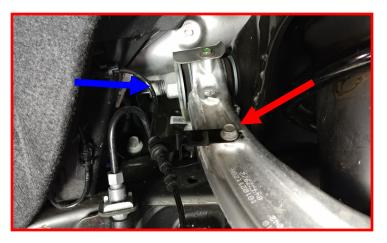
Loosen but do not remove the upper ball joint nut. Strike the ball joint boss with a dead blow hammer to dislodge the taper. Remove the upper control arm from the knuckle. Let the knuckle hang out of the way. Take care to not over extend the brake line and ABS wires.
