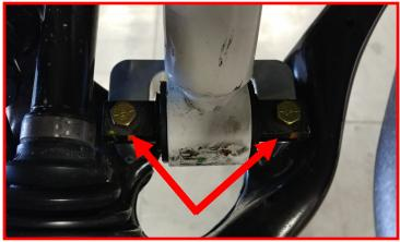
Use the jack and raise the lower control arm up. Guide the upper ball joint into the knuckle and re-attach using the factory hardware. Torque to 65 ft-lbs.
