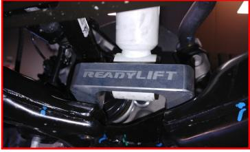
Install the provided 3/8" bolts, washers and nuts from the strut side facing down. You may need to use a pry bar or an assistant to help guide the strut into place while dropping the bolts through the lower control arm. Torque to 45 ft-lbs.
