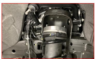
Install the supplied lower strut spacer between the strut cross pin and the lower control arm
