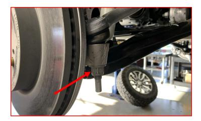
Install the ABS sensor harness and brakeline bracket to the knuckle.
