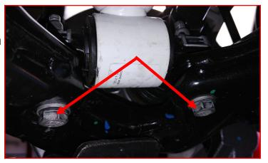
Remove the (3) top strut mounting nuts located on top of the strut tower and discard the nuts. Remove the strut assembly from vehicle.
