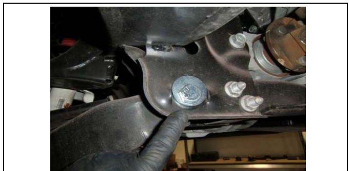
12. Install the provided alignment cam bolts as shown.
