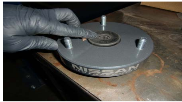
22. Insert the sleeve through the top and bottom bushings.
