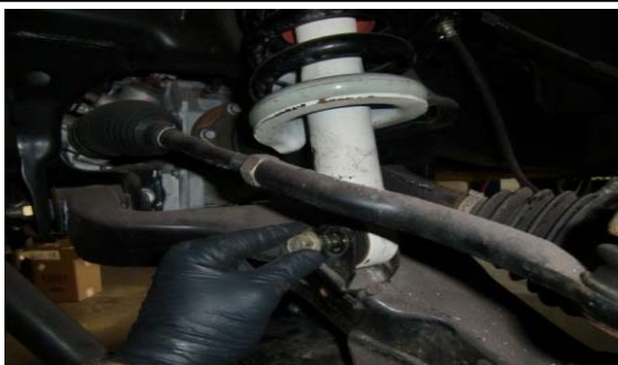
27. Reinstall the lower strut to the lower control arm with OE hardware.
