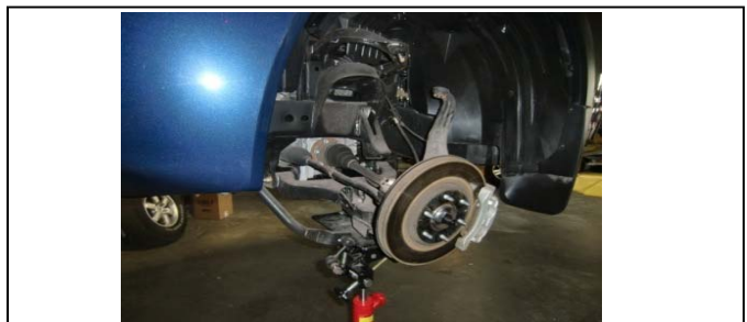
10. With the lower control arm supported, disconnect the upper control arm from the spindle, then carefully lower the jack to drop the suspension. Remove the strut from the vehicle.
