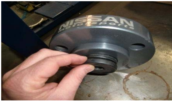
21. Install the new center sleeve with the OE bushings as shown.
