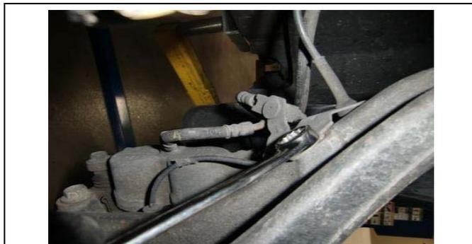
3. Remove the ABS/ brake line bracket from the backside of the spindle.
