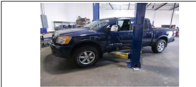
1. Measure from the ground to the fender well, across the center of the wheel, for all four wheels. Record the data in the space provided on page two. Place the vehicle on level ground and lift it up from the frame.
