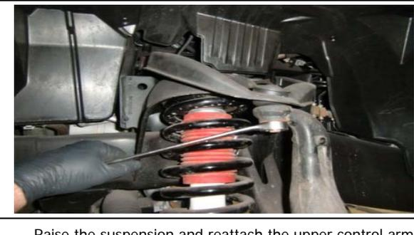
28. Raise the suspension and reattach the upper control arm to the spindle using the OE hardware.
