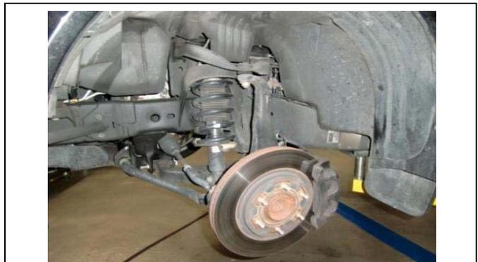
2. Remove the front wheels from the vehicle.
