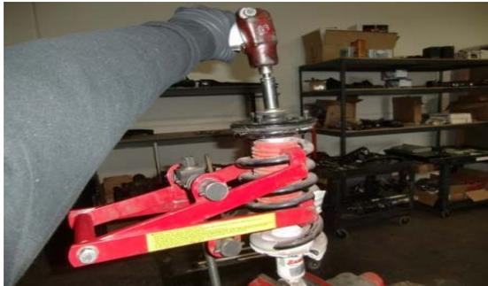
17. Carefully remove the upper coil-over center nut.
