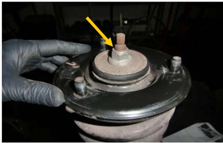
If necessary, use penetrating oil on the center stud to help with nut removal on next step.
