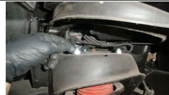
26. Install the upper strut with provided nuts.
