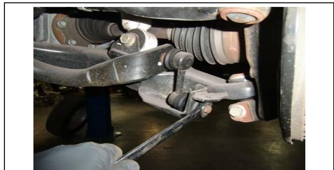
4. Disconnect the sway bar end links from the sway bar on both passenger and driver sides.
