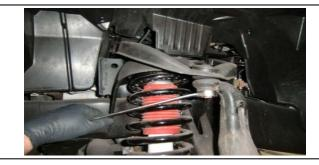
Raise the suspension and reattach the upper control arm to the spindle using the OE hardware. 28.
