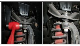
Separate the upper ball joint from the spindle. A hammer may 9. be necessary.
