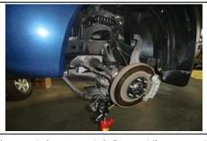
With the lower control arm supported, disconnect the upper control arm from the spindle, then carefully lower the jack to drop the suspension. Re
