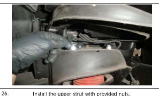
Install the upper strut with provided nuts.
