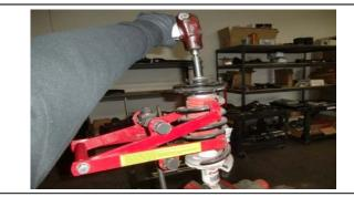
17. Carefully remove the upper coil-over center nut.
