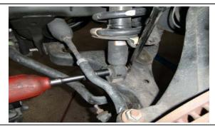
6. Remove the nut and bolt from the lower strut mount.
