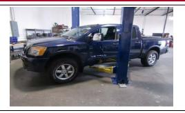
Measure from the ground to the fender well, across the center of the wheel, for all four wheels. Record the data in the space provided on page two. Place the vehicle on level ground and lift it up from 1.
