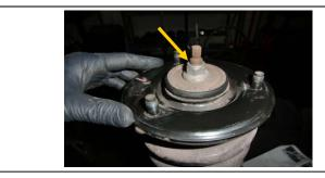
If necessary, use penetrating oil on the center stud to help with nut 15. removal on next step.
