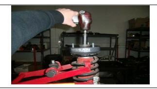
24. Tighten the OE hardware to spec.
