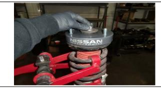
23. Reinstall the upper assembly back on top of the strut.
