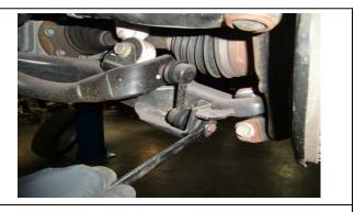
Disconnect the sway bar end links from the sway bar on both 4. passenger and drivers sides.
