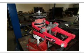
16. Use a coil spring compressor to safely remove the spring from the strut.
