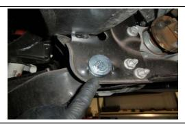
12. Install the provided alignment cam bolts as shown.
