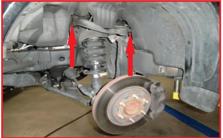
Remove **ABS wire** from their steel brackets. Remove the **brake lines** from the knuckle. Remove the cotter pin from the upper ball joint, and loosen but don not remove the **ball joint nut**.
