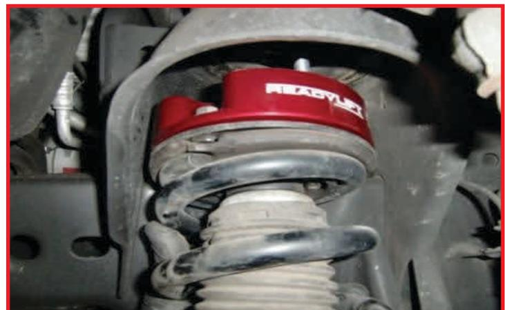
Raise the LCA, reconnect the strut to the lower control arm using the factory hardware. Do not tighten at this time.
