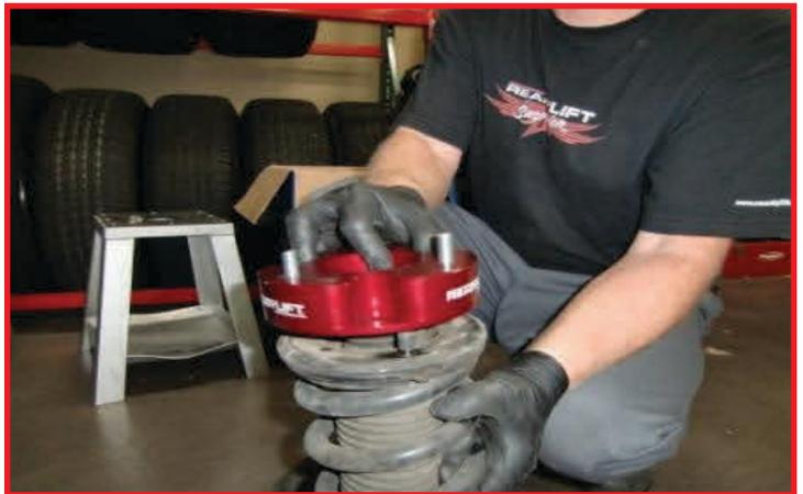
The strut assembly will be clocked 180 degrees for reinstallation.
