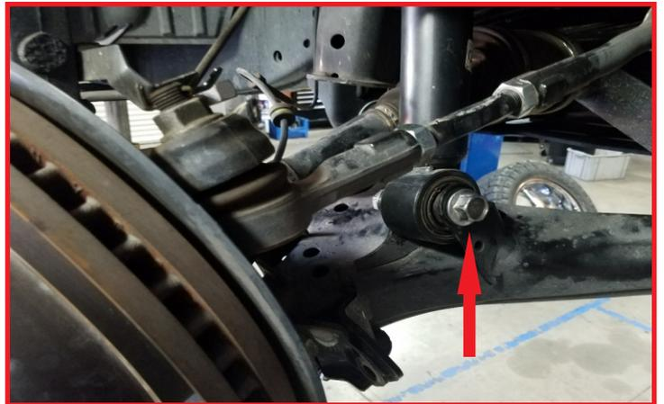
Support the lower control with a suitable jack, With the upper ball joint nut loose, strike the ball joint boss with a dead blow hammer to dislodge the taper (indicated from the red arrow). Once the taper is dislodged remove the upper ball joint hardware, and separate the UCA from the knuckle.
