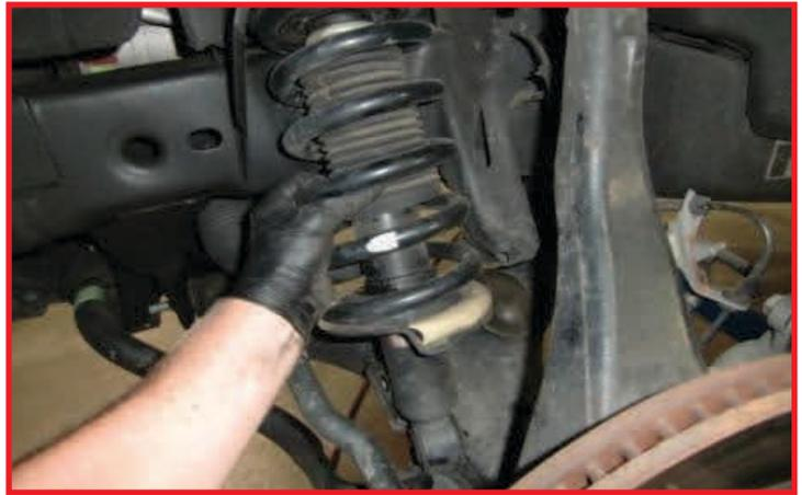
Attach the ReadyLIFT strut extension to the top of strut using the **factory hardware** to fasten, Torque to **30 ft lbs**.
