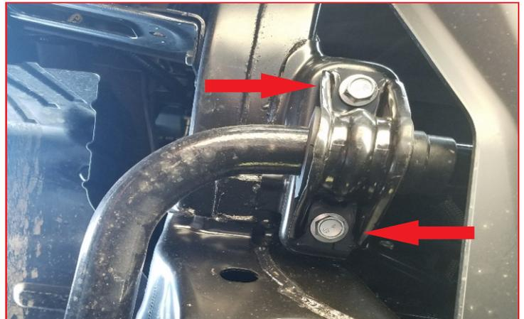
Remove the lower strut mounting hardware.
