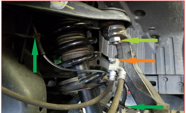
Remove the three upper strut mounting nuts.
