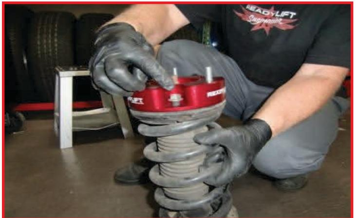
Reattach the strut to the strut tower in the vehicle using provided **M10 flange nut**. Do not tighten at this time.
