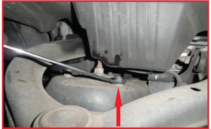
Disconnect driver and passenger side sway bar from the frame rails, and let hang out of the way.
