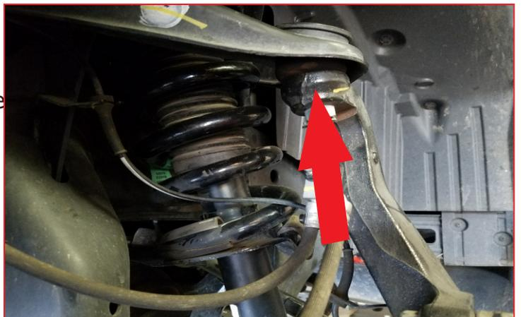
Loosen but do not remove the lower control arm (LCA) hardware at the frame. Lower the LCA while supporting the knuckle and remove the strut from the vehicle. Take care to not over extend or stretch the ABS-rubber brake lines. Adjust as necessary.
