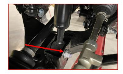
Remove the four (4) upper strut bolts.
