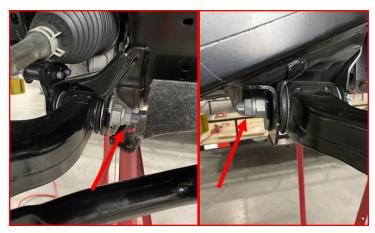
Remove lower strut bolt and remove strut from vehicle.
