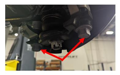
Remove lower control arm to strut bolt.
