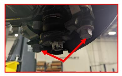
Install the sway bar end link to the lower control arm using factory hardware.
