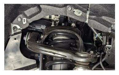
On the strut top mount, measure and mark 3/8'' from the top of each stud.
