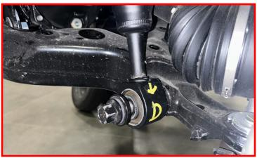
Install the tie rod into the knuckle.
