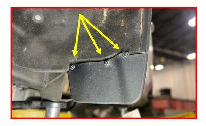
Remove the two screws securing the back of the mud flap.
