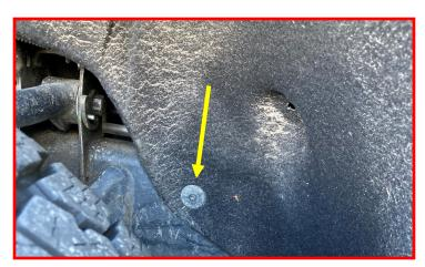
Install the fender liner using the two previously removed screws.
