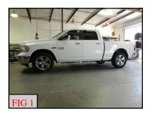
Park vehicle on a clean flat surface and block the rear wheels for safety. Engage the parking brake.
