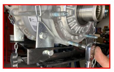
Install the supplied transfer clocking ring. It may be necessary to rotate the ring until all the mounting holes align.
