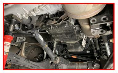
The transmission mount is attached with (4) bolts. Remove the (2) bolts located at the rear of the mount and retain the factory hardware.
