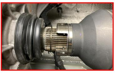
Mark the driveshaft to pinion flange location. Remove the rear driveshaft hardware from the flange. Let hang out of the way. Retain the factory hardware.
