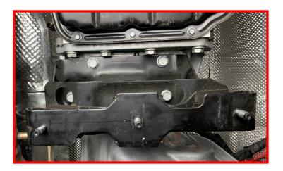
Install the provided transmission mounting plate using the factory transmission mount nuts. Do not tighten at this time.
