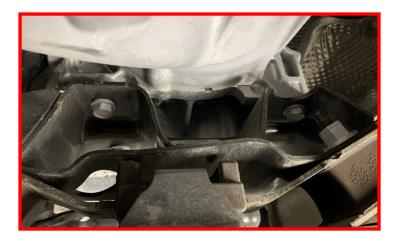
Tighten the transmission mount bolts. Torque the hardware to 40 ft-lbs.
