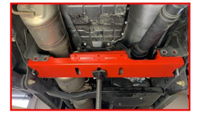
Using the factory transmission crossmember hardware, install the driver side from front to rear.
