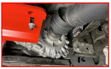
Slide the dust boot back over the front output splines.
