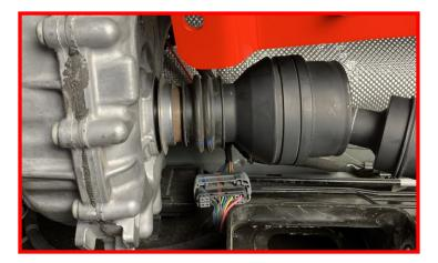
Install the supplied clamp onto the dust boot and joint housing.
