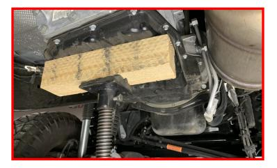
Ensure the transfer case is free of any other harness clips and the harnesses are not wrapped, hung on or caught on any part of the transfer case.
