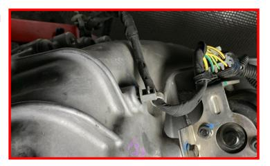
Install the transfer case harness retaining clip located on the top of the transfer case.
