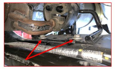
Raise the DPF with a suitable jack and remove the (2) passenger transmission crossmember bolts. Retain factory hardware.
