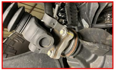
Carefully remove the larger clamp on the front driveline dust boot. Slide the boot back to gain access to the retaining clip.
