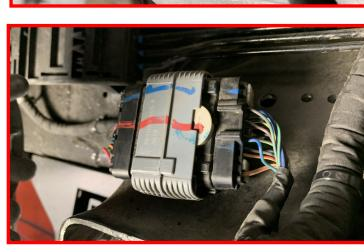
Install the harness connector onto the relocation bracket.
