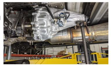
Using a transmission jack, remove the transfer case from the vehicle. Set aside.
