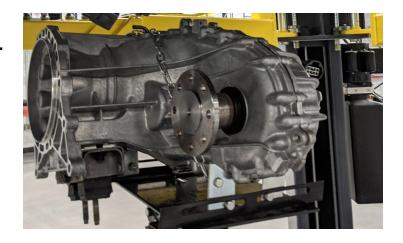
Install the ReadyLIFT Transfer Case Clocking Ring into the transmission using the provided M10 x 35mm socket cap bolts. Place some thread-locker on each bolt before installation. Using a star pattern, torque bolts to 40 ft-lbs.
