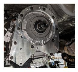
Re-install transfer case using the provide M10-1.5 x 35mm Hex Bolts. Place some thread-locker on each bolt before installation. Using a star pattern, torque bolts to 40 ft-lbs.
