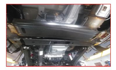
Support transfer case with jackstand near the output shaft. Remove factory cross member and discard. Retain the 4 factory bolts and nuts that hold the transfer case on the outsides.
