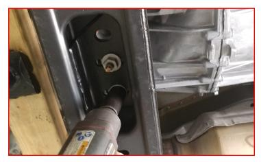
With the transfer case still supported, remove the front and rear drive shafts from the vehicle. Retain factory driveshafts and hardware.
