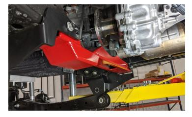
Install the provided M12-1.5 nuts and washers to the bottom transmission studs and torque to 65 ft-lbs.
