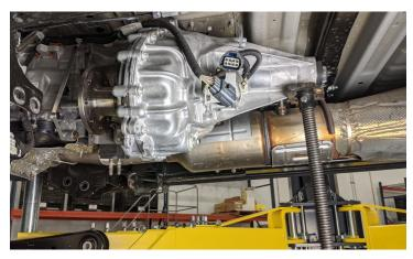
Line up the ReadyLIFT Transmission Crossmember and put the factory bolts through on each side. Install factory nuts onto the bolts and torque to 40 ft-lbs.
