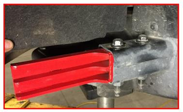
Install the fender liner retaining clip above the rear anti-intrusion beam.
