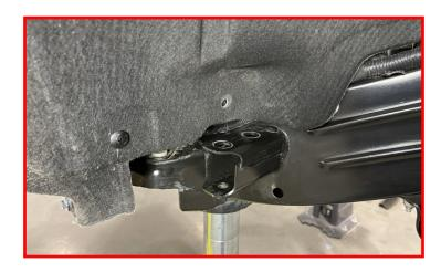
Install the replacement Rear Anti-Intrusion Beam using the factory hardware.
