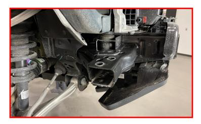
Install the replacement Front Anti-Intrusion Beam using the factory hardware.
