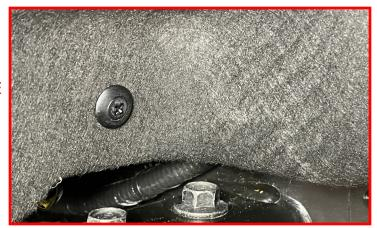
Remove the (2) factory M12 bolts and discard the cut factory beam.
