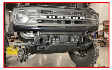
Remove the (2) factory M12 bolts and discard the cut factory beam.
