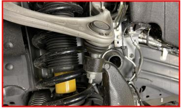
Remove the upper control arm pivot bolt.
