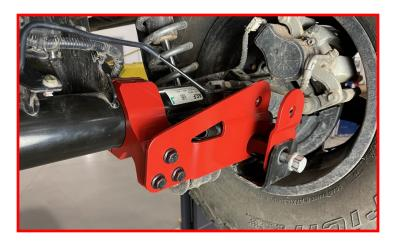
Install the rear track bar into the track bar bracket using the supplied M16 x 90mm hex flange head bolt.
