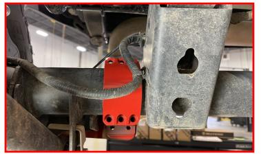
Align the (3) mounting hole on the track bar bracket to the front track bar clamp.
