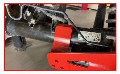
Install the rear track bar clamp on to the front side of the axle and aligned with the front clamp.
