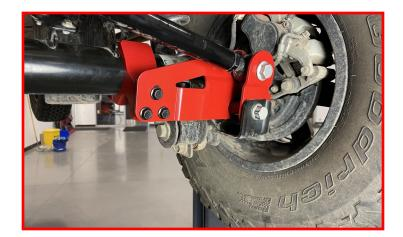
Install the wheels and lower the vehicle to the ground. Torque the lug nuts to the wheel manufacturers specs. Jounce the vehicle to settle the suspension to the new ride height.
