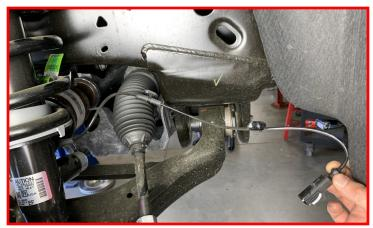
Install the (2) retaining clips that secures the CCD solenoid harness to the frame.
