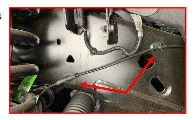
Connect the CCD solenoid harness connector.
