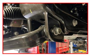
Tighten the top strut nuts.
