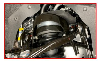
Raise the lower control arm up and guide the lower strut studs into place.
