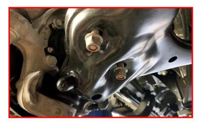
Loosen and remove the lower control arm pivot bolts.
