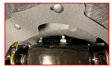
Remove the lower strut nuts.
