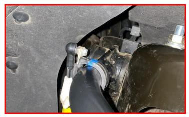
Using the factory nuts, install the strut assembly into the strut tower.
