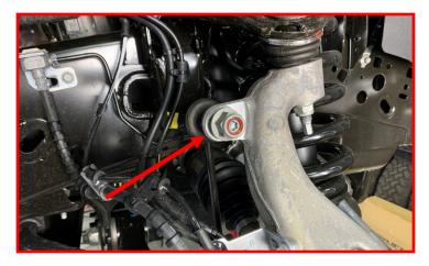
With everything tightened and torque to the specified specifications, install front tires and lower vehicle. Torque the lower control arm hardware to 200 ft-lbs
