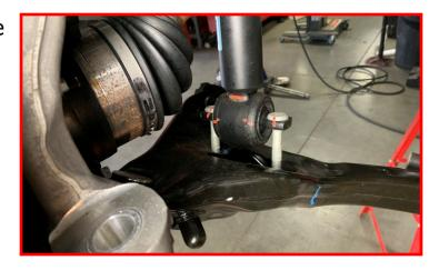
Continue to raise the lower control arm up until you are able to install the factory lower strut nuts.
