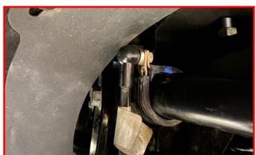
Install the threaded end of the ball socket to the clamp and tighten with OE nut.
