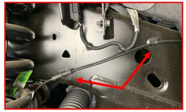
Disconnect the CCD solenoid harness connector located on top of the frame behind the inner fender liner.
