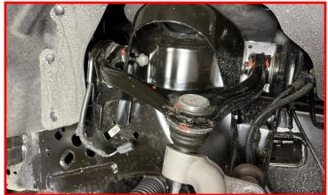
Install the supplied upper control arm in the factory orientation.
