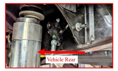
On the radius arm, remove the headlight leveling bracket.
