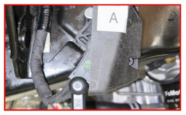
Remove the Bump stop and extension from the frame. Install ReadyLIFT 1" Bump Stop extension on top of the original Bump Stop Extension using the provide M8 x 95mm bolt and washer.
