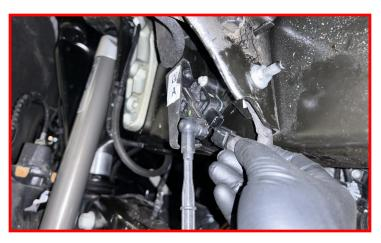
Remove retaining clip from bracket.
