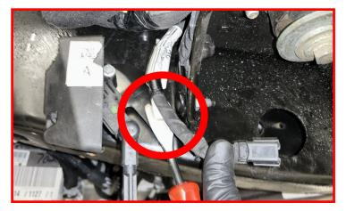
Remove the nut holding the leveling sensor link to the radius arm.
