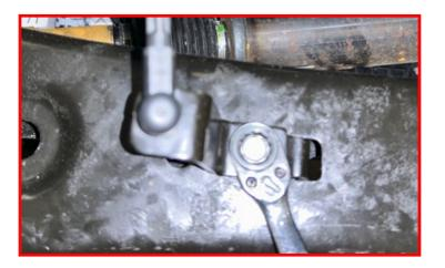
Install ReadyLIFT headlight leveling bracket onto radius arm using factory hardware. The slot in the bracket should be toward the rear of the vehicle.
