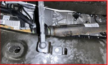
Remove headlight leveling bracket and sensor from frame.
