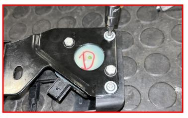
Remove headlight leveling sensor from factory bracket.
