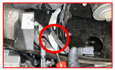
Remove headlight leveling bracket from radius arm.
