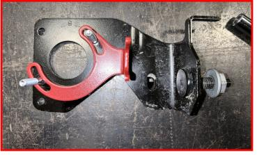
Install the factory headlight leveling sensor onto the bracket using factory nuts. Ensure that the sensor arm is placed inside the "Y" shape of the ReadyLIFT bracket.
