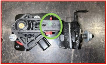
Install the bracket assembly onto the frame using factory hardware. Bracket should be installed on the opposite side of the body mount wall from factory location, with the bolts pointing toward the inside of the vehicle. Bracket assembly should be inside the body mount.
