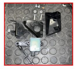
Remove sensor arm from sensor.
