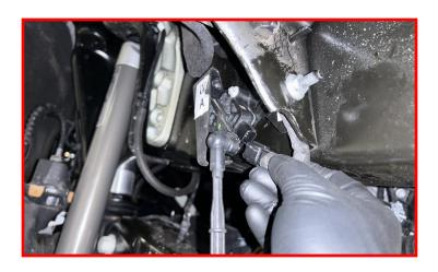
Remove retaining clip from bracket.
