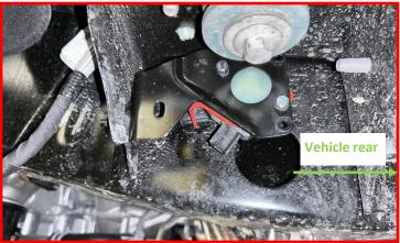
Plug the connector into the headlight leveling sensor.
