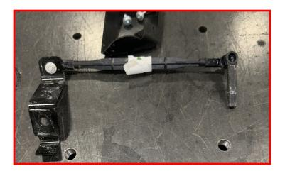
Install ReadyLIFT headlight leveling delete bracket in between factory headlight bracket and factory headlight level sensor with the supplied M5 bolts pointing up.
