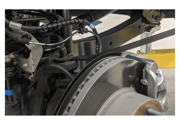
6. Install ReadyLIFT 68-2500CB caster bushing by inserting into around factory ball joint stud and sliding into the hole previously occupied by factory caster slug. Slot on caster slug should be pointing outboard from centerline of vehicle.
