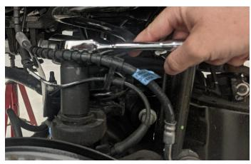
5. Pull upwards on factory caster bushing to remove from vehicle. A pry bar or pickle fork may be necessary to assist with removal. Be careful not to damage factory coating on knuckle.
