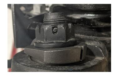
8. Re-insert factory cotter pin into the ball joint and castle nut.
