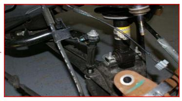
Attach the upper ball joint to the knuckle using the provided hardware. Torque to 85 ft-lbs. DO NOT use an impact.
