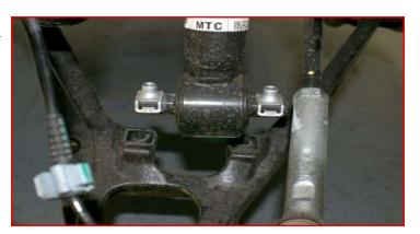
Remove the upper strut mount at the frame. Remove the strut from the vehicle.
