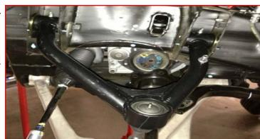
Raise the lower control arm and install the lower strut using the factory hardware. Torque to 45 ft-lbs.
