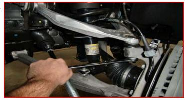
Strike the upper ball joint boss to release the taper.
