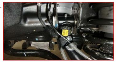
Attach the ABS wire to the frame rail with the factory clip. Re-connect the electrical connector.
