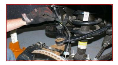
Remove the brake line bracket from the upper control arm and frame rail.
