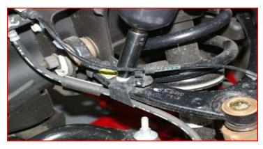
Remove the sway bar end links from the sway bar and lower control arm.
