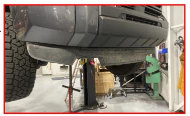
Install the supplied jack point spacer using the supplied 3/8 self threading bolts.
