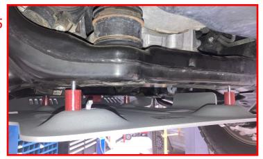
Pull the skid plate toward the rear of the vehicle and torque the (6) skid plate bolts.
