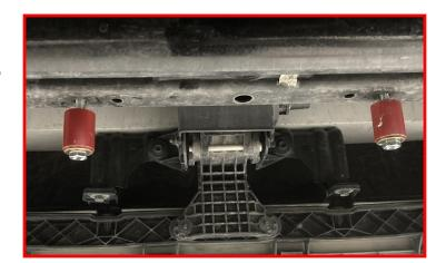
Raise the skid plate into position by using the two slotted holes at the front of the skid plate.
