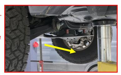
The AAS will automatically retract when the vehicle is started and placed into either drive or reverse.
