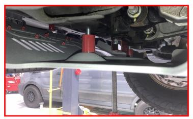
Raise the skid plate slightly and install the rear most spacers followed by the M8-1.25 bolt and washer.
