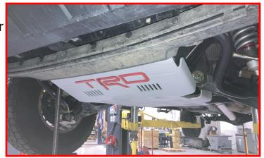
With everything tightened and torqued to the specified specifications, lower vehicle.
