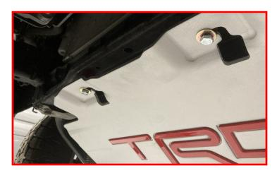
Raise the skid plate slightly and install the two spacers at the middle of the plate (between the plate and the frame) followed by the M8-1.25 bolt and M8 washer.
