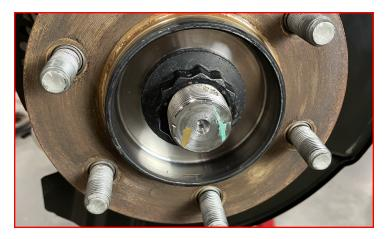
With the aid from a helper, pull hub assembly forwards toward the front of the vehicle.
