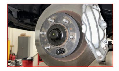
Remove the cotter pin and nut retainer.
