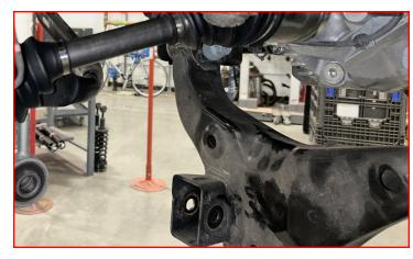
Apply a small amount of medium duty thread locker to the factory lower ball joint bolts.
