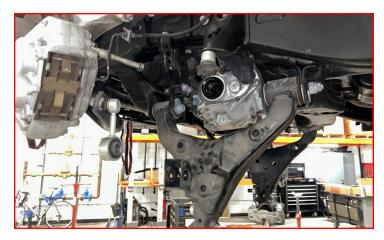
Locate the replacement axle assembly. The axle are etch with the part number on the shaft. The 68-52420CVL is the Left (driver) side and will be the shorter of the two.
