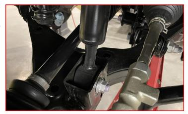
Install the sway bar end link onto the lower control arm.
