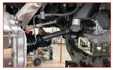
Install the supplied axle nut.
