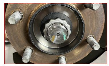
Remove the axle nut and release the axle from the hub.
