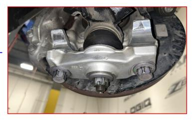
Raise the lower control arm enough to insert the factory lower strut bolt and nut. Install from front to rear.
