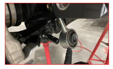
Ensure the hub is supported with a suitable jack.
