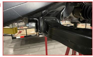
Remove the lower shock bolt.
