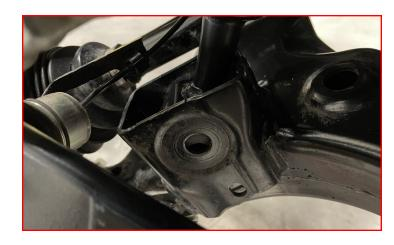
Carefully swing the lower control arm down and out of the way.
