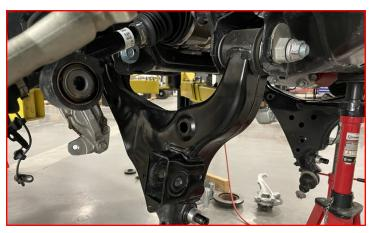
Remove the CV axle dust shield.
