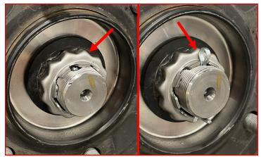
Install the factory axle nut dust shield.
