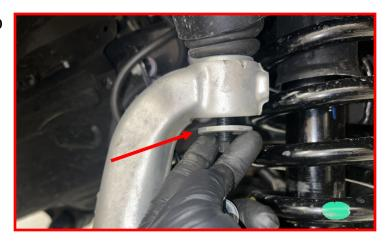
Install the supplied M12 flange nut onto the ball joint.
