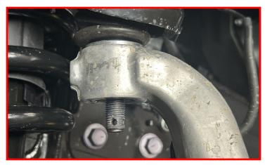
Remove the upper control arm pivot nut.
