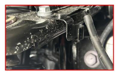
Remove the retaining clip from the upper control arm ball joint nut.
