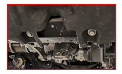
Find the threaded holes in the rear crossmember. M8 bolts will be installed into the rearward, outboard threaded holes. (Avoid installing in the forward, inboard holes).
