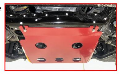
Install the provided M8 bolts and washers to the front side of the skid plate. Felt dust shield should be installed on the outside of the skid plate.
