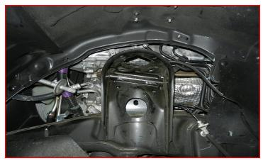
Install the replacement upper control arm to the frame using the factory hardware, and supplied large washer to the inside edge of the control arms. Do not tighten at this time.
