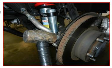
Remove the ABS sensor and harness from the knuckle and hang out of the way.
