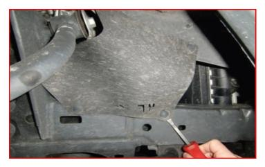
Remove the upper control arm from the frame. Take care as the upper control arm bolt is very long and has to pass through the engine compartment by some electrical harness and coolant lines. It is best to remove the lines off the inner fender well on the passenger side to gain enough access to pass the bolt forward. (Strut shown removed for clarification. Will be removed in a later step.)
