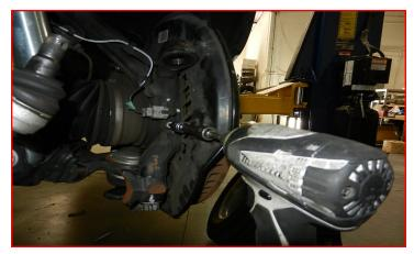
Remove the brake line bracket from the upper control arm.
