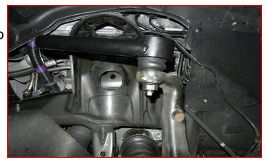
Remove the outer tie rod end using the factory castle nut.
