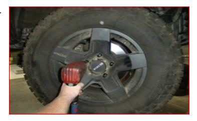
Jounce the front suspension to settle the vehicle to ride height. Center the lower control arm cams and torque to 100 ft-lbs (final torque to be done by alignment professional), upper control arm to 150 ft -lbs, lower strut hardware to 125 ft-lbs, and the sway bar end link hardware to 50 ft-lbs. Connect the vehicle power source at the ground terminal on the battery.
