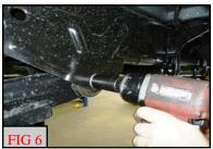
Install radius arm drop bracket for the side that you are working on using the factory hardware. Do not tighten at this time. Repeat steps for the opposite side. (Fig 8)
