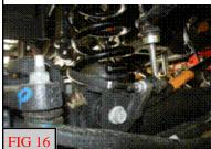
Reinstall the sway bar to the frame using the factory hardware. Torque to 45 ft-lbs.
