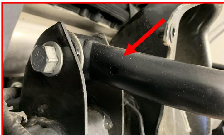
Install the strut to the frame rail using the provided **M10 - 1.25 flange nut**. Do not tighten at this time.
