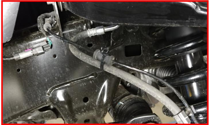
Install the sway bar to the frame rail using the **factory hardware**. Torque to **35 ft-lbs**.
