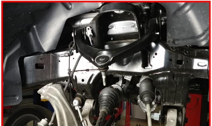
Remove the upper control arm from the frame.
