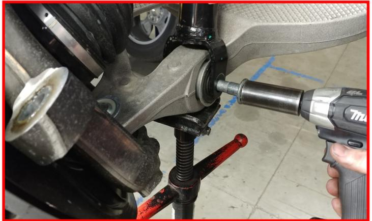
Remove the upper strut hardware from the frame.
