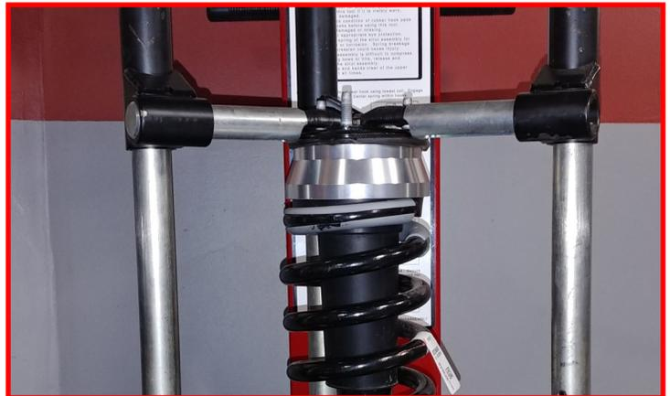
Locate the ReadyLIFT top strut extension and install using the **factory hardware**. Torque to **30 ft-lbs**.
