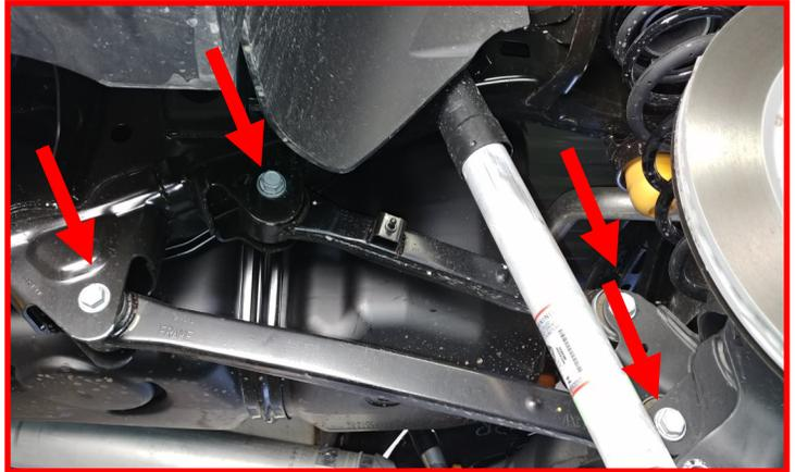
Loosen but do not remove the track bar hardware at the frame and axle ends.
