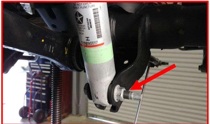
Locate the upper sway bar end link and brake line bracket mount on the frame rail.
