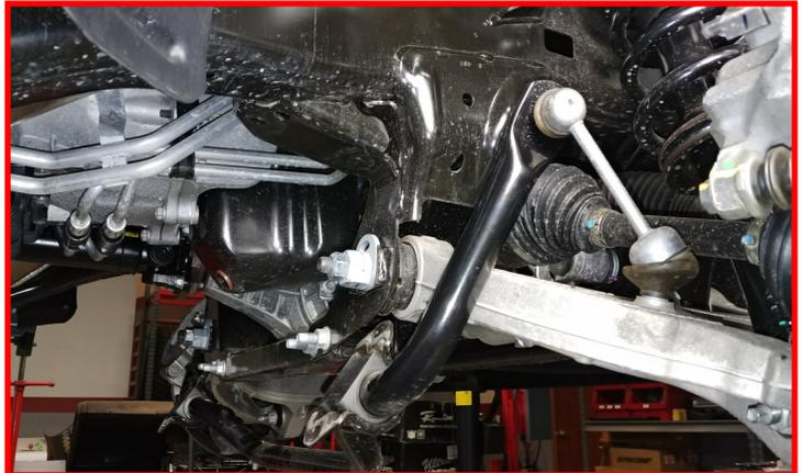
Support the lower control arm with a suitable jack.
