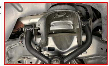
To determine the correct side arm, there is a plugged hole on the back tube of the near the rearmost pivot. Be sure this faces the rear of the vehicle.
