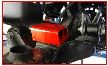
The driver side you will use the bolt hole on the left inside hole of the bump extension. This will line up with the hole in the axle pad. The forward mounting hole is slotted to line up with the axle pad hole. Once the inside bolt is lined up, install the front bolt, washer, and nut.
