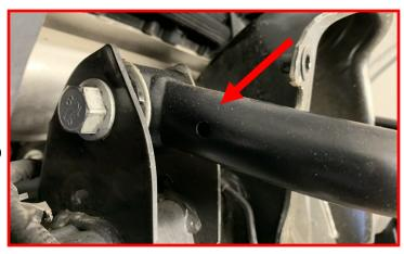
Install the strut to the frame rail using the provided M10 - 1.25 flange nut. Do not tighten at this time.
