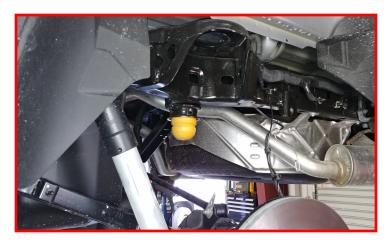
The rubber isolator has two locating nipples on it. Use a suitable cutting device, remove these flush with the isolator.
