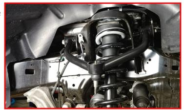
Raise the lower control arm up until you can install the lower strut hardware. Do not tighten at this time.
