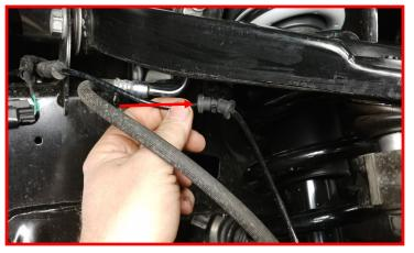
Remove the outer tie rod from the knuck-le.
