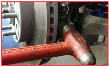
Remove the upper ball joint from the knuckle.
