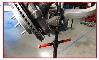
Remove the lower strut mounting hardware. Lower the control arm down while supporting the knuckle. Be mindful of the ABS and brake lines to not over extend them.
