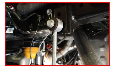
Remove the upper sway bar end link and brake line bracket at the frame rail.
