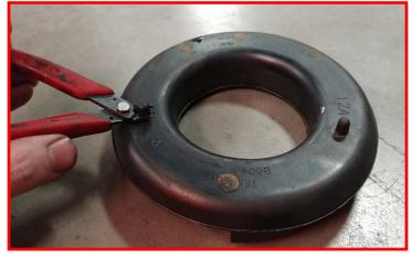
Install the ReadyLIFT bump stop extension to the axle pad using the provided 1/4" bolts, washers, and nuts. Torque to 5 ft-lbs. The bump stop extensions are universal for both sides of the axle.
