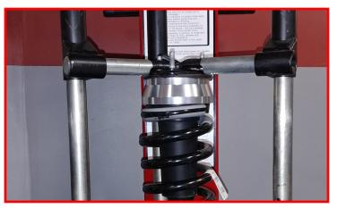
Locate the ReadyLIFT top strut extension and install using the factory hardware. Torque to 30 ft-lbs.
