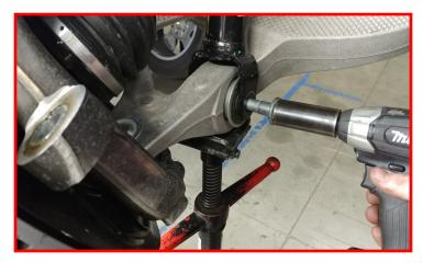
Remove the upper strut hardware from the frame.
