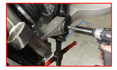
Attach the upper control arm ball joint to the knuckle using the provided hardware. Install the nut spacer, then the castle nut.
