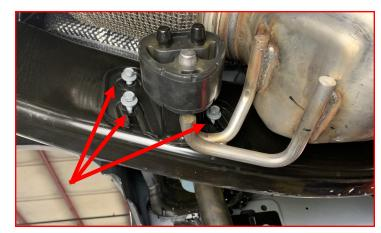
Rotate the axle and install the radius arms into the drop brackets using the provided 18mm, washers and c-lock nuts. Do not tighten at this time.
