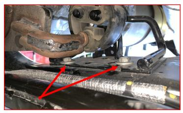
Raise the DPF with a suitable jack and remove the (2) passenger transmission crossmember bolts. Discard factory hardware.
