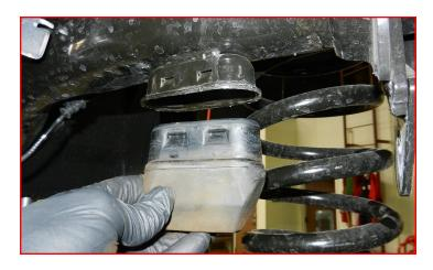
Install extended bump stops. To aid in install, lube the mounting end with a soap and water mix.
