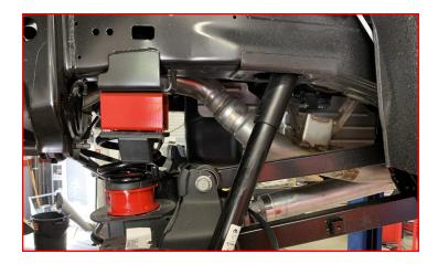
Install the shocks onto the axle using factory hardware. Do not tighten at this time.
