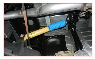
Install the rear wheels and lower vehicle to the ground. Torque the lug nuts to the wheel manufacturer specs. Torque the upper shock stem to 30 ft-lbs, lower shock bolts to 90 ft-lbs, sway bar end links to 45 ft-lbs, bump stop extension to 30 ft-lbs, parking brake bracket 10 ft-lbs, track bar mounting bolts to 100 ft-lbs and the upper and lower control arm bolts to 200 ft-lbs.
