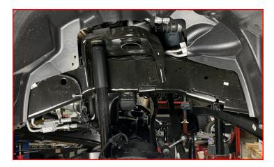
Using an appropriate cutting tool remove the alignment tab. It is necessary to trim the tab off of the coil spring isolator for reinstall.
