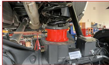
Remove factory shock bushing and washer. Be sure to retain the bushings and washers.
