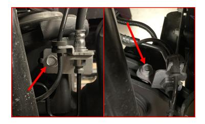
Locate the brake line/ABS bracket on the inside of the frame rails and remove.
