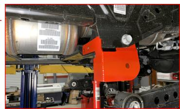
Install supplied M16 bolts and washers through crossmember and radius arm drop bracket mounting holes and attach with supplied washers and lock nuts. Installing them in the opposite direction from factory (From front to rear). This will aid in removal if service needs to be performed.
