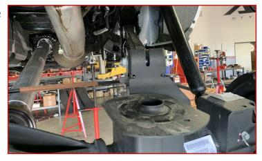
Install the coil spring with coil spring spacers and isolators. Raise the axle high enough to keep springs and spacers in place.
