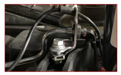
Install the ABS sensor harness and brake line bracket to the axle.
