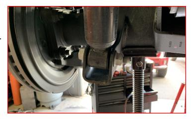
Remove the rear bump stops. Retain factory hardware.
