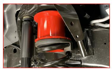
Install the supplied shock extensions onto the shock using 14mm bolts, washers, clock nuts. Raise the axle enough to install the extension onto the axle using the factory hardware. Do not tighten factory hardware at this time.
