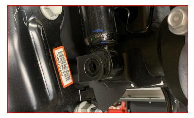
Remove the sway bar mounting hardware from the frame. Lower sway bar and let hang out of the way.
