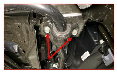
Loosen track bar mounting bolts at both the axle and the frame. Do not remove at this time.
