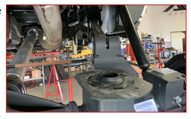
Install the coil spring with coil spring spacers and isolators. Raise the axle high enough to keep springs and spacers in place.
