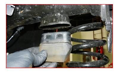
Install extended bump stops. To aid in install, lube the mounting end with a soap and water mix.
