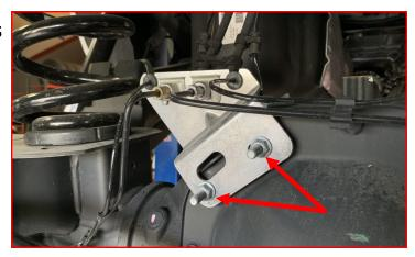
Loosen but do not remove the upper and lower control arm bolts on the axle and the frame pockets.
