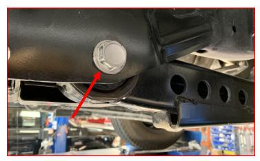
Mark the driveshaft to pinion flange location. Remove the front driveshaft hardware from the flange. Let hang out of the way. Retain factory hardware.
