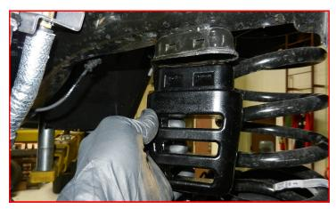
Remove the frame side track bar mounting bolt and lower the track bar out of the way.
