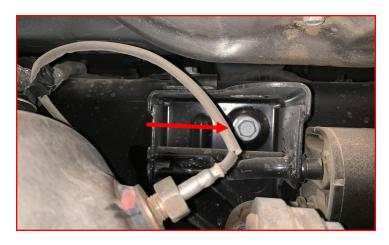
Remove the (2) Diesel Exhaust Fluid (DEF) tank crossmember exhaust hanger mounting bolts.
