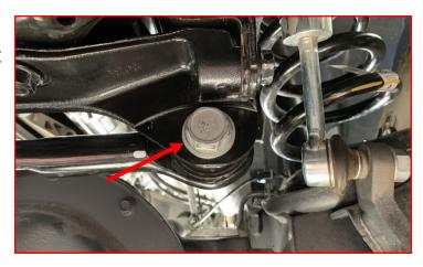
Lower the axle enough to remove the front springs. Make sure to not over extend the brake/ABS lines.
