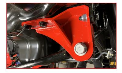
Install the ABS sensor harness and brake line bracket to the radius arm.
