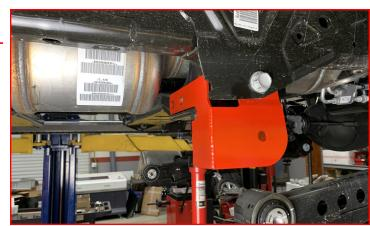
Install crossmember mounting bolts, installing them in the opposite direction from factory. This will aid in removal if service needs to be performed.
