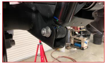
Install the sway bar end links using M12 x 70mm bolts, washers, and c-lock nuts. Insure the fender washer is installed on the outside of the bushing.
