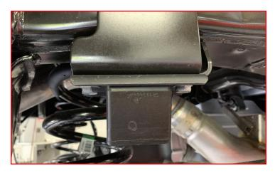
Loosen the track bar at the axle and frame mounts but do not remove.
