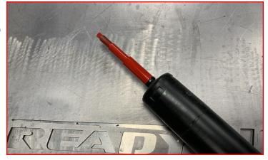
Install factory shock washer and bushing on to the shock extension in a factory orientation.
