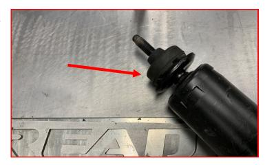
Using a liberal amount of thread locker, install the supplied shock extensions on to the top of the shock shaft.
