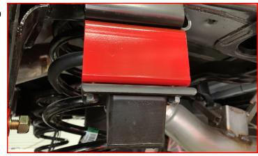
Install the shocks onto the frame using factory hardware.
