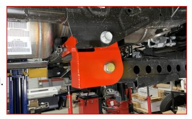
With the axle fully supported, remove the lower shock bolts. Retain factory hardware.
