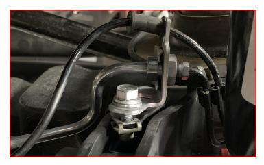
Install the ABS sensor harness and brake line bracket to the axle.
