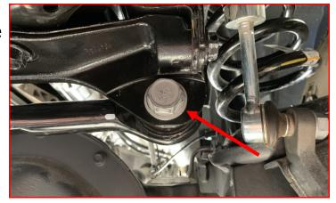
Remove the (5) factory mounting bolts from the factory track bar bracket and remove from vehicle. Retain factory hardware.
