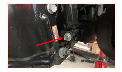
Place a jack under the axle for support. Remove the radius arm bolts. Retain factory hardware.
