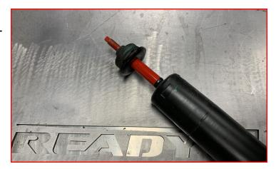
Install the bump stop and extensions onto the frame using factory hardware. Install the bump stop using 3/8" bolts, washers, and c-lock nuts.
