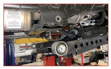
Support the transmission crossmember with a suitable jack stand. Working on one side at a time, Loosen and remove two transmission crossmember bolts.
