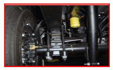
Slightly loosen but do not remove the passenger side u-bolts. Remove the driver side u-bolts completely and discard.
