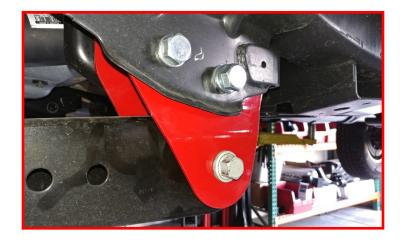
Remove the brake line bracket at the frame. Remove the brake line bracket at the axle.
