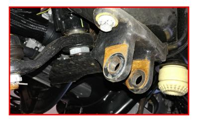
Install the ReadyLIFT track bar bracket to the frame using factory hardware. Torque to 95 ft-lbs. Install the track bar to the ReadyLIFT bracket using factory hardware. Do not tighten at this time.
