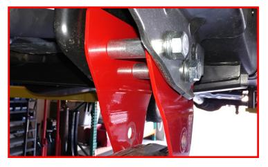
Rotate the axle until you can line up the radius arms into the ReadyLIFT drop brackets. Install using factory hardware. Do not tighten at this time.
