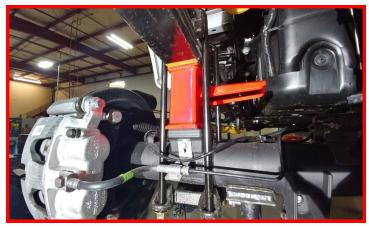
If equipped with a 2 piece driveline, remove the bolts holding the carrier bearing to the frame. Install the ReadyLIFT carrier bearing spacer between the carrier bearing and frame using 7/16" bolts, washers and nuts. Torque to 50 ft-lbs.
