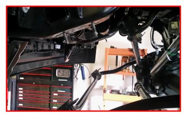
Remove the track bar from the factory bracket. Remove the factory track bar bracket from the frame.
