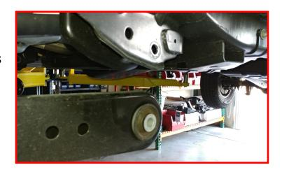
Install the ReadyLIFT radius arm drop brackets into the frame using M18 x 130mm bolts, washers, crush sleeve, and nuts. Do not tighten at this time.
