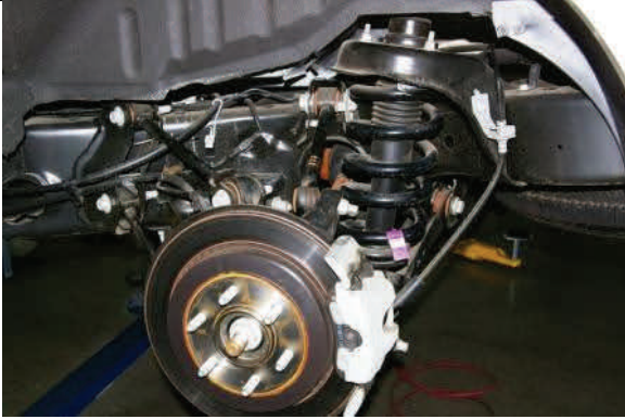
Raise rear of vehicle remove wheels/tires, support frame
