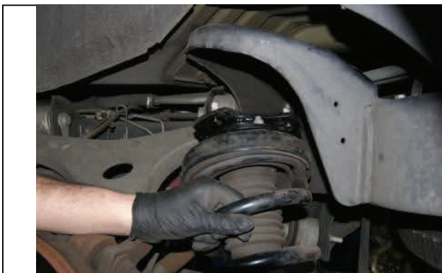
Reinstall strut with new nuts and reverse removal steps
