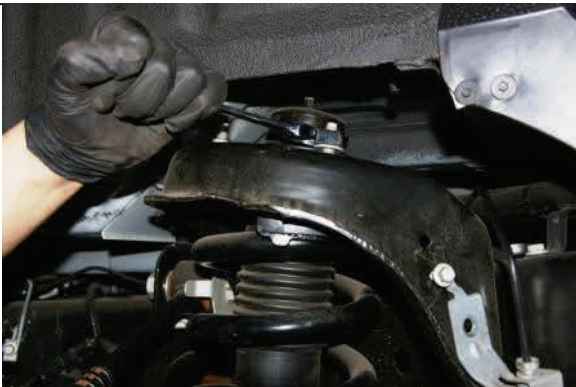
Remove upper strut mounting hardware.
