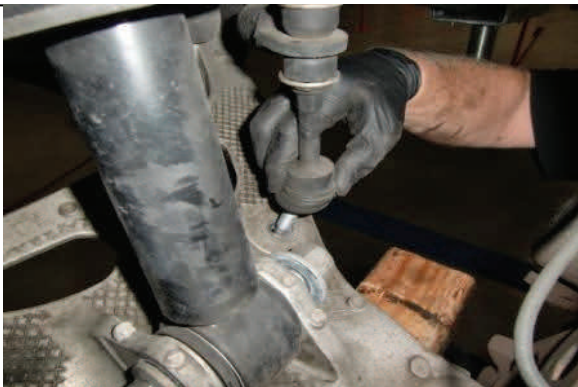
Reconnect lower sway bar endlinks and torque to spec.
