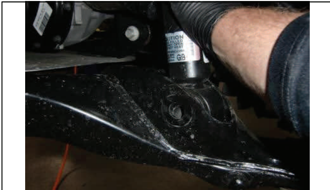
Push down suspension and reinstall lower strut bolt and nut.
