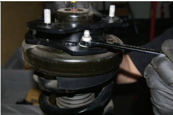
Attach upper strut extension with OE hardware.
