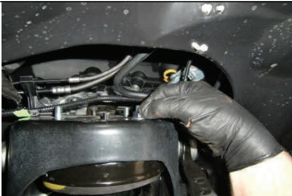
Use provided hardware to re-attach top of strut to vehicle.
