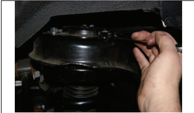
Tighten upper strut mounting hardware
