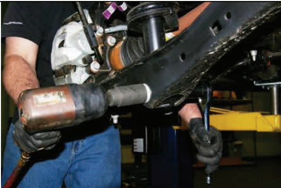
Remove lower strut mounting hardware.
