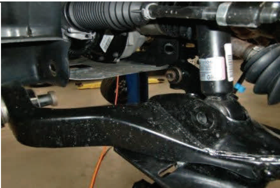
With jack, lower control arm from frame pockets.
