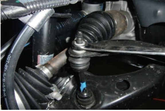
Disconnect upper sway bar end links.
