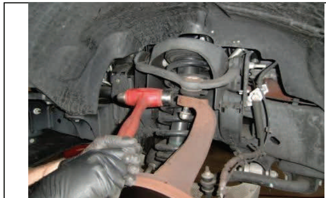
Carefully strike spindle as shown to separate ball joint.
