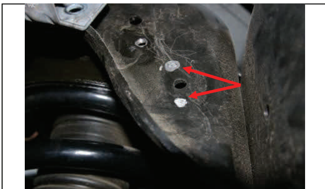
Use 3/16 drill and reuse OE mounting bolt to reattach.
