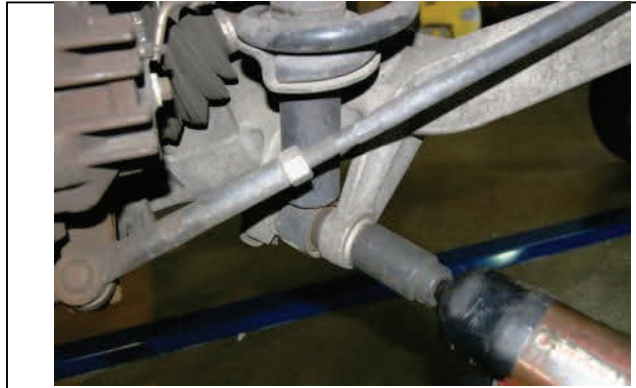
Remove lower strut mounting hardware.
