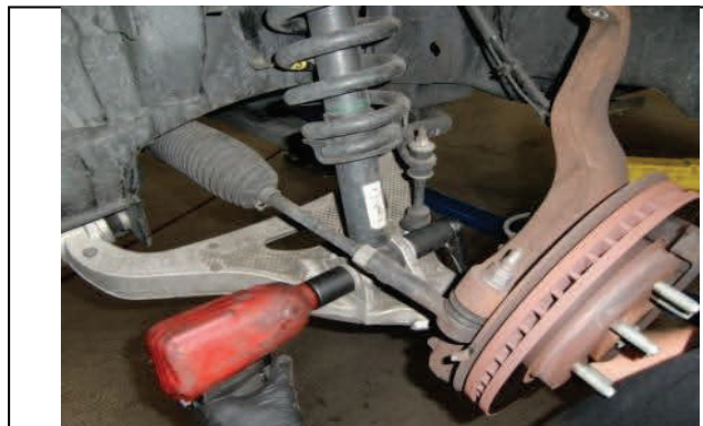
Loosen lower strut bolt/nut and remove.
