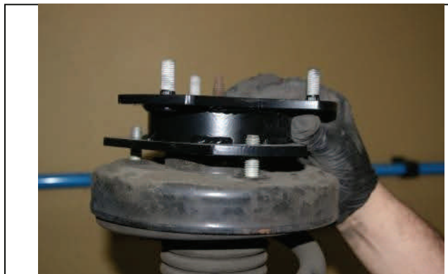
Install strut extension with OE hardware and tighten
