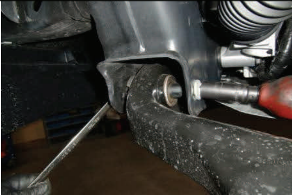
Loosen and remove front lower control arm bolt and nut
