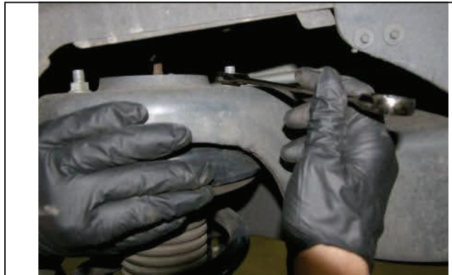
Remove upper strut mounting nuts
