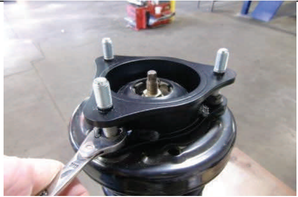
Attach strut extension spacer with OE hardware and tighten.
