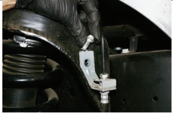
Unbolt brake line bracket from coil bucket.
