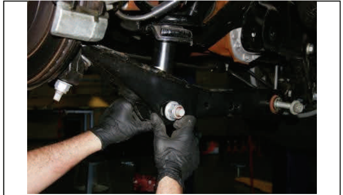
Reinstall lower strut mounting bolt. Tighten later.
