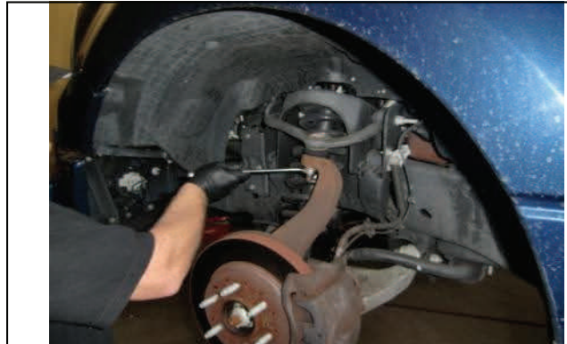
Loosen upper ball joint nut, but do not remove.
