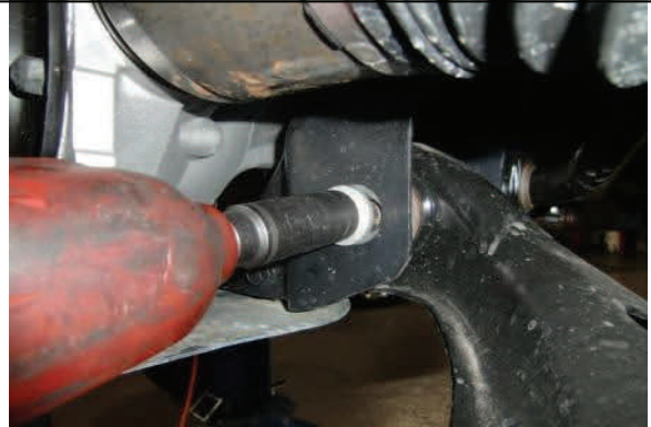
Loosen and remove rear lower control arm bolt and nut.
