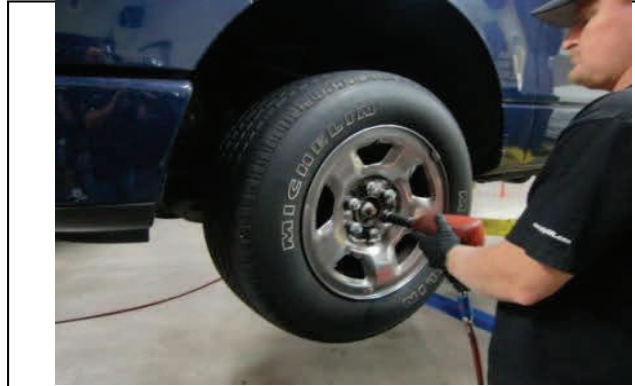
Lift vehicle securely and remove wheels/tires.
