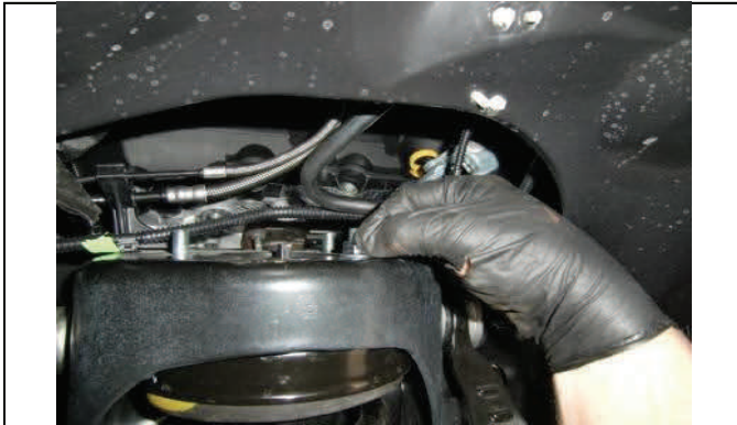
Rotate strut 180 degrees and reinstall with new hardware.
