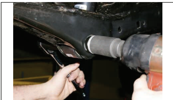
Torque lower shock/control arm bolts with vehicle on ground.
