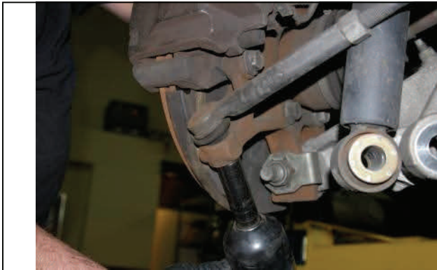
Remove tie rod nut and carefully strike spindle to break loose
