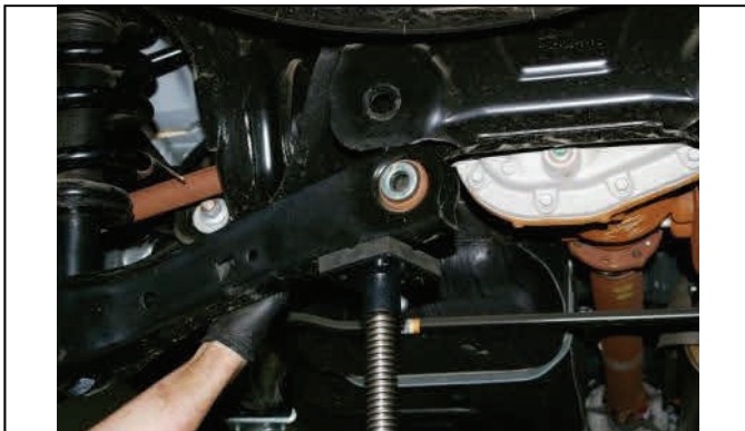
Use jack to raise lower control arm and connect with OE bolt.
