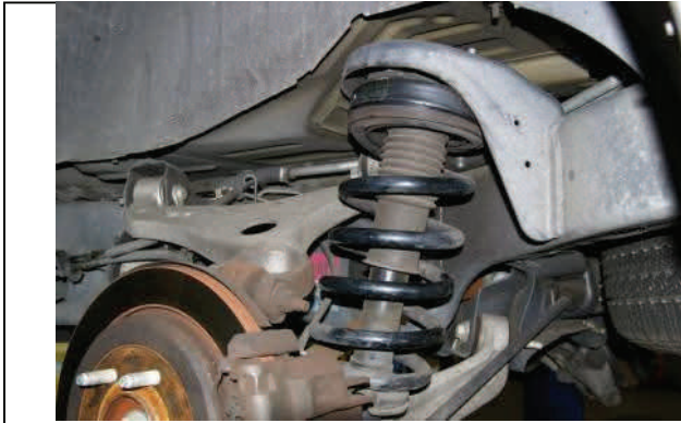
Remove rear wheels/tires and support frame.
