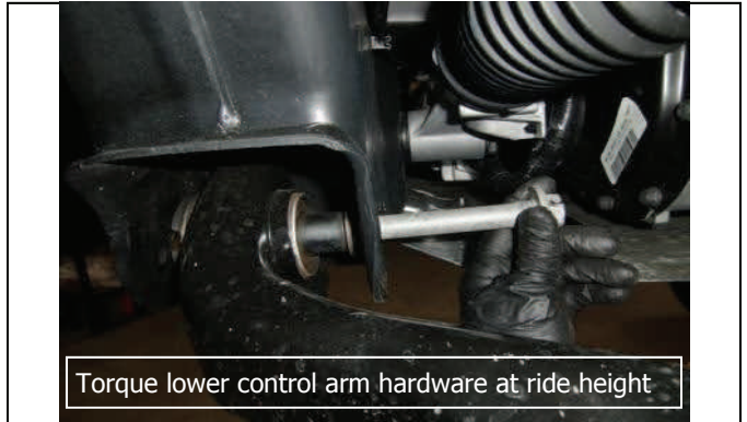
Lift lower control arm into position and reinstall bolts.
