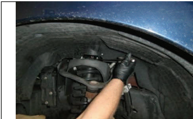
Loosen upper strut mount nuts.
