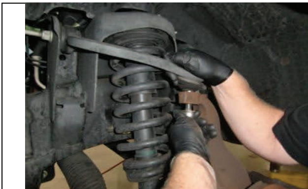
Pull down and remove upper ball joint nut.
