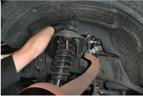
Remove top strut mount nuts and remove assembly.
