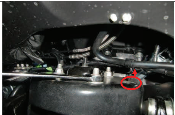
Pry ABS line clip out and remove upper strut mounting nuts.
