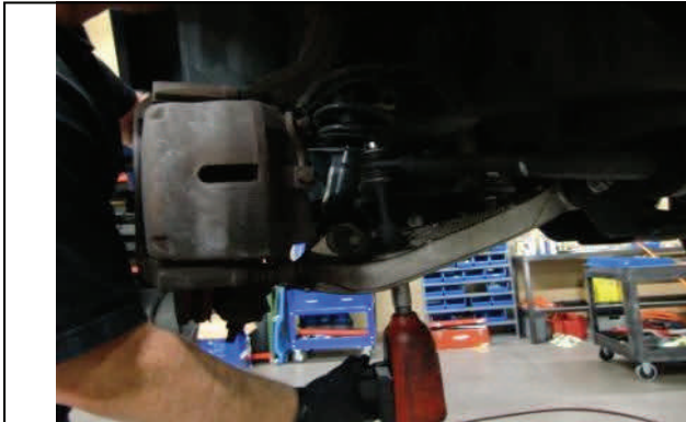
Remove lower sway bar endlink hardware.
