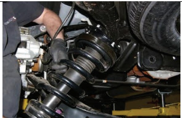
Reinstall strut assembly in vehicle with new nuts.
