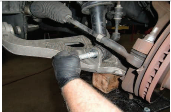
Reconnect lower strut mount and torque to spec.
