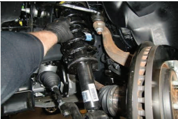
Remove strut assembly from vehicle
