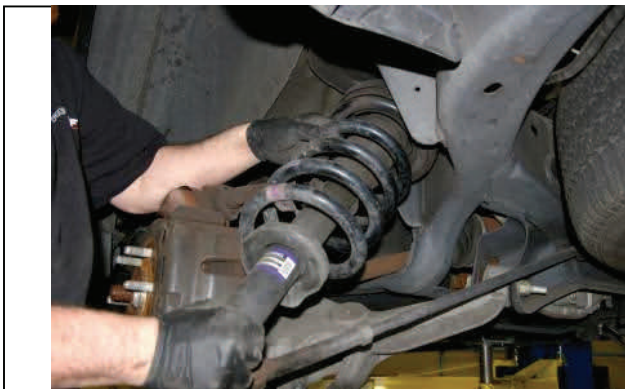
Remove strut assembly from vehicle
